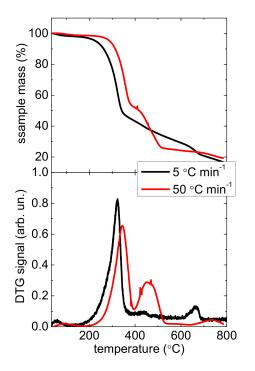
**Figure 3.** Mass loss (upper panel) and corresponding derivative curve of a RDF. Thermogravimetric analyses have been performed from 30 °C up to 800 °C on a Perkin–Elmer STA6000 under inert atmosphere (N<sub>2</sub>, flux 40 mL/min), applying two different heating rates: 5 °C/min and 50 °C/min.
