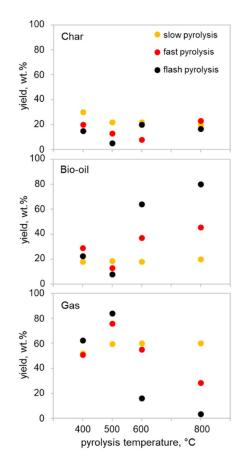
**Figure 2.** Product yields obtained from pine wood pyrolysis at different temperatures under slow, fast, and flash pyrolysis conditions (adapted from [52]).
