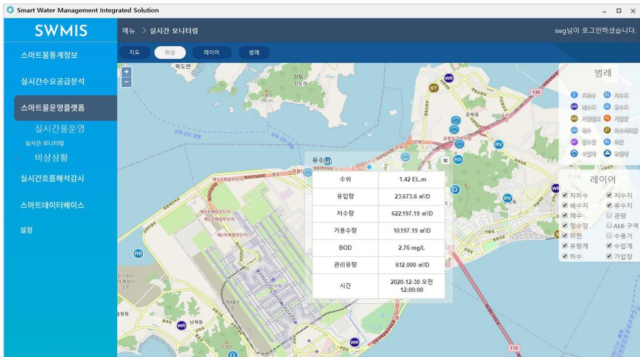
**Figure 14.** Smart water management integrated solution dashboard: Real-time WDN operation by SWG-DSS (water level, inflow, outflow, storage volume, available quantity, BOD, management flow, and time).
