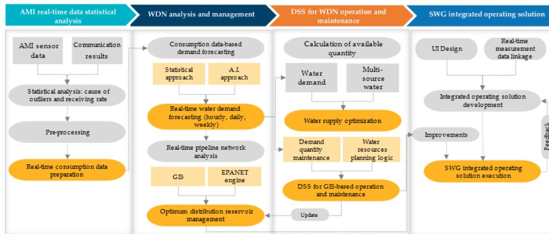
Figure 10. Procedure for developing SWG integrated operation solution.
