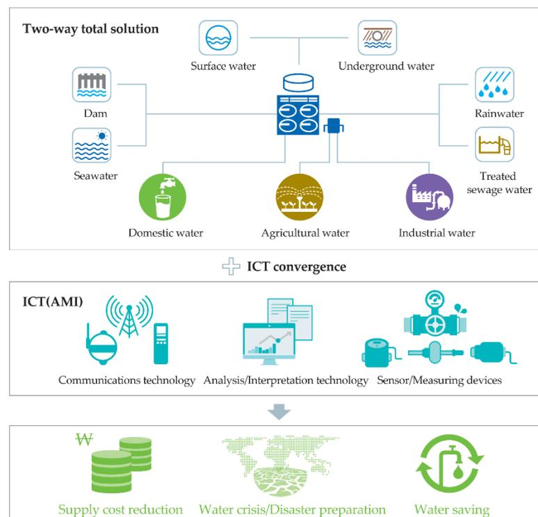
**Figure 1.** Representative diagram of SWG architecture.
