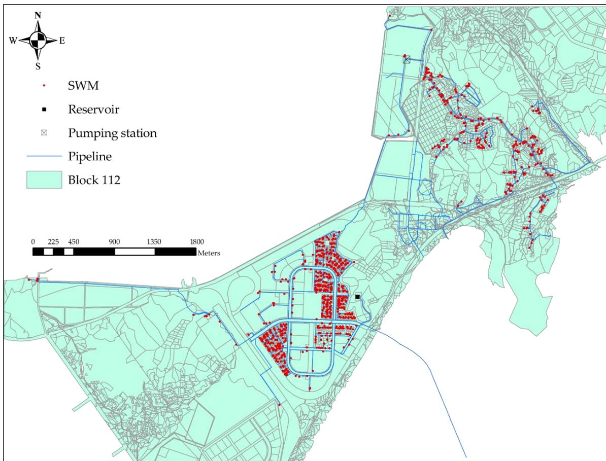
**Figure 7.** Deployment of smart water meter in Block 112.
