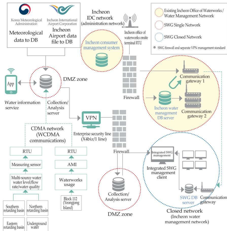
**Figure 9.** Block diagram for integrated management of bi-directional smart water information.
