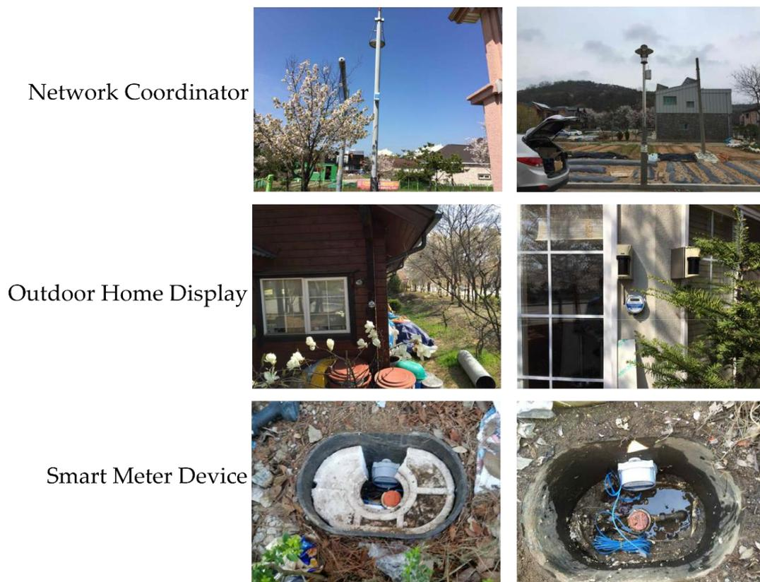
**Figure 8.** Setup of AMI network device.
