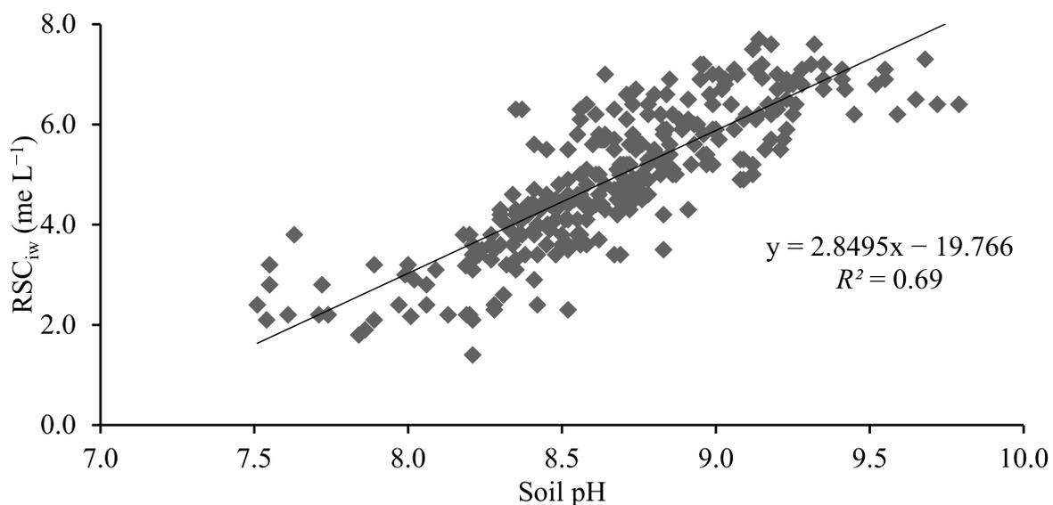
**Figure 2.** Relationship between irrigation water residual alkalinity and estimated soil sodicity across the sampled locations ( $n = 308$ ).
