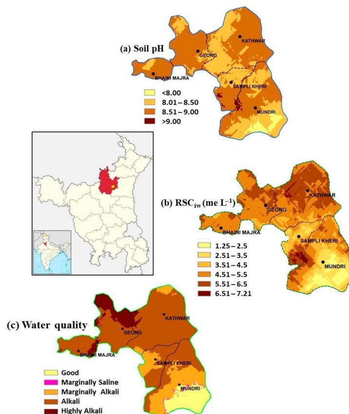
**Figure 1.** Maps showing the extent and distribution of (a) sodic soils, (b) residual alkalinity in irrigation water, and (c) water quality status in the study area.
