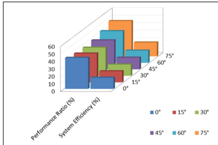
**Figure 8.** Performance ratio and system efficiency in several tilt angles.
