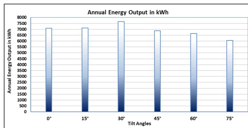
**Figure 10.** The yearly energy output of different tilt angles.
