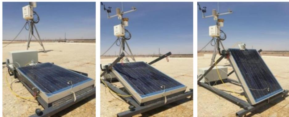
**Figure 3.** Field measurements of an off-grid PV system with different tilt angles ( $0^\circ$ ,  $30^\circ$ , and  $60^\circ$ ).
