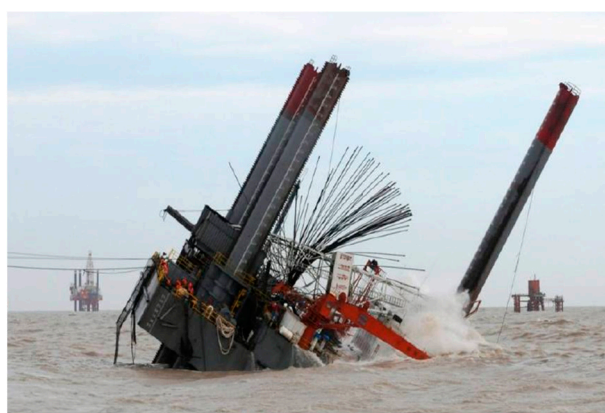
Figure 2. ShengLi Well Workover Platform III overturning accident [3].
