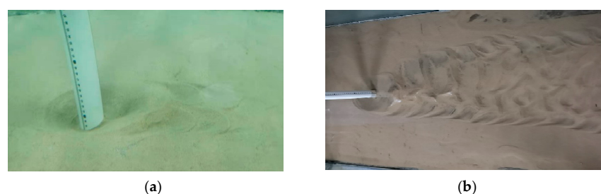
Figure 7. Pictures of scour holes and scour forms under combined waves and current (Run C1). (a) After 15 min, (b) After 3 h.
