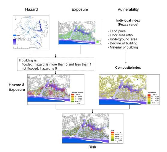
**Figure 4.** Procedure of calculating flood risk by combing methods of physical and index-based risk assessment.
