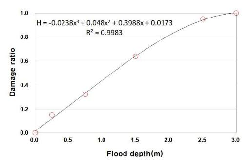
Figure 5. Flood depth-damage ratio curve of building for hazard calculations.
