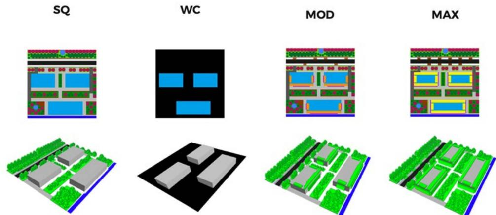
**Figure 6.** Example of greening scenarios of an urban standard typology (SQ = status quo of greening; WC = worst case (no greening); MOD = moderate case; Max = maximum case) (Green4Cities/GREENPASS, 2018).
