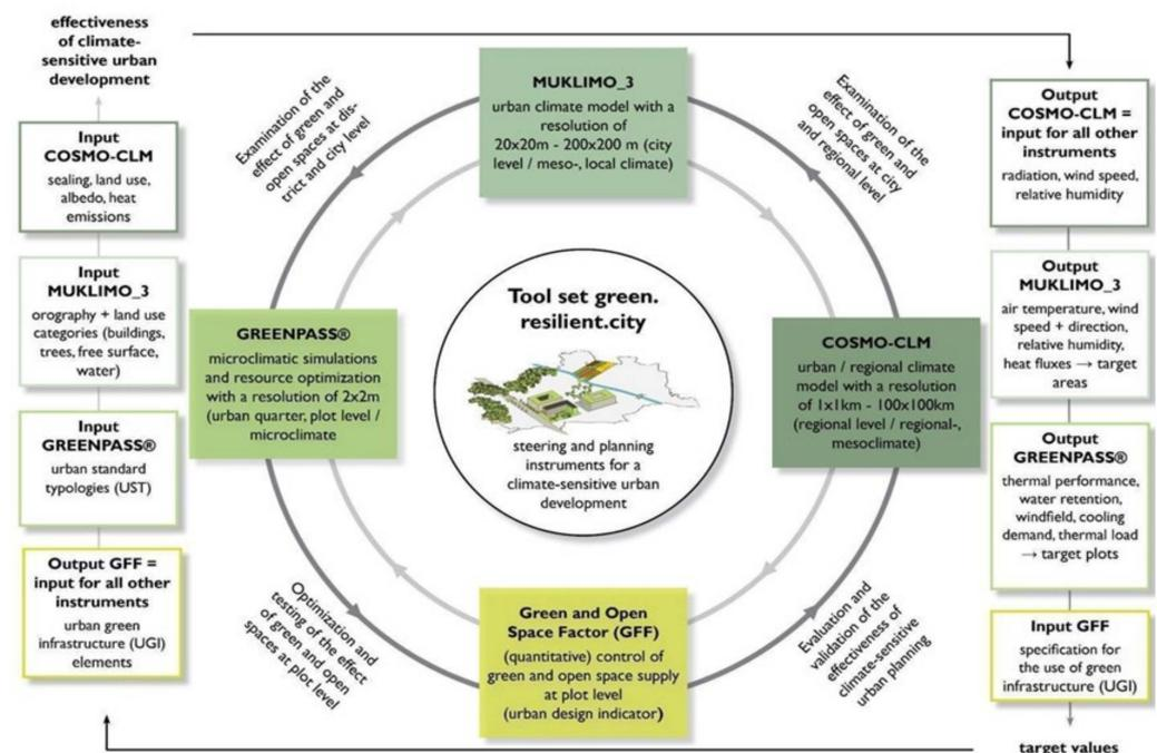
**Figure 14.** The multi-scale Green.Resilient.City toolset as steering, evaluation and optimisation investment at various climate and planning levels (ILAP/GRC project consortium).
