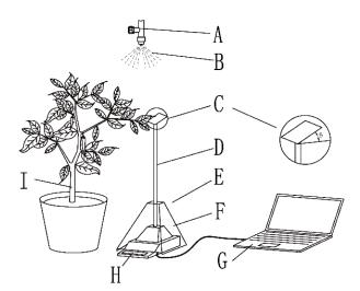
Figure 3. Droplet retention measurement device: (A) spray nozzle; (B) droplet clouds; (C) object stage; (D) connecting rod; (E) insulating shell; (F) electronic balance; (G) computer; (H) balance readings; (I) plants.
