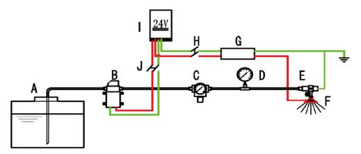
**Figure 2.** Schematic diagram of electrostatic spraying system: **(A)** tank; **(B)** diaphragm pump; **(C)** pressure gauge; **(D)** pressure regulator; **(E)** electrode; **(F)** fan nozzles; **(G)** electrostatic generator; **(H)** switch of electrostatic generator; **(I)** DC power supply; **(J)** switch of diaphragm pump.
