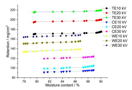
**Figure 8.** Retention at different water contents of three crops. TE denotes the retention of tomato leaves under electrostatic conditions, CE the retention of pepper leaves under electrostatic conditions, and WE the retention of winter wheat leaves under electrostatic conditions; 10, 20, and 30 kV represent electrostatic voltages.
