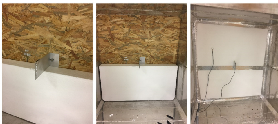
Figure 15. Sample no. 2. anchor without thermal bridge interruption.
