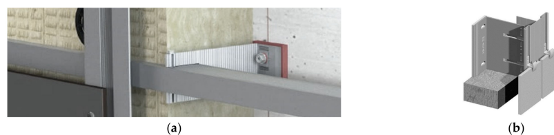
Figure 2. Example point thermal ventilation of the façade. (a) Aluminum anchor with a plastic pad; (b) method of attaching the tile [30].
