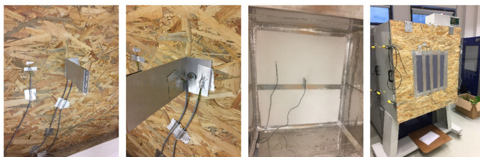
Figure 16. Temperature sensors applied to sample.
