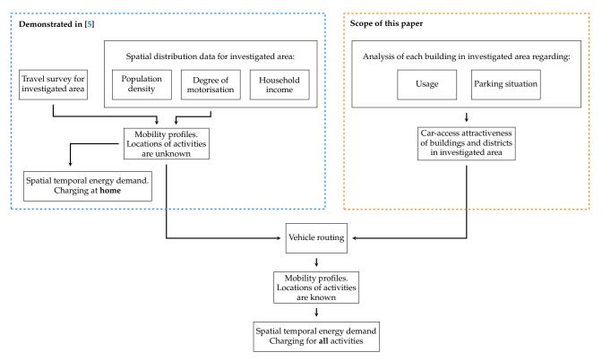
Figure 2. Method for estimating the spatial and temporal energy and power demand from the electrification of private ICEVs.
