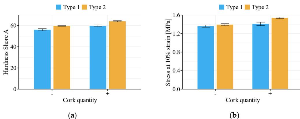
**Figure 2.** Results of cork analysis: (a) Hardness Shore A; (b) Static compression stress at 10% strain.
