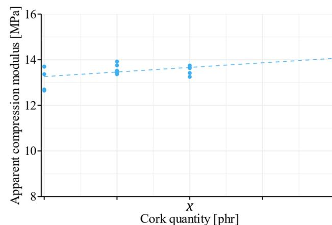
**Figure 9.** Experimental data and regression model: static behavior.
