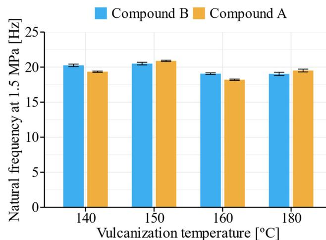
**Figure 8.** Results of vulcanization temperature analysis: natural frequency at 1.5 MPa.
