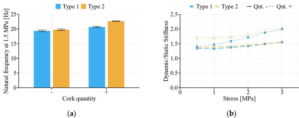
**Figure 3.** Results of cork analysis: (a) Natural frequency at 1.5 MPa; (b) Ratio between dynamic and static stiffness at different loads.
