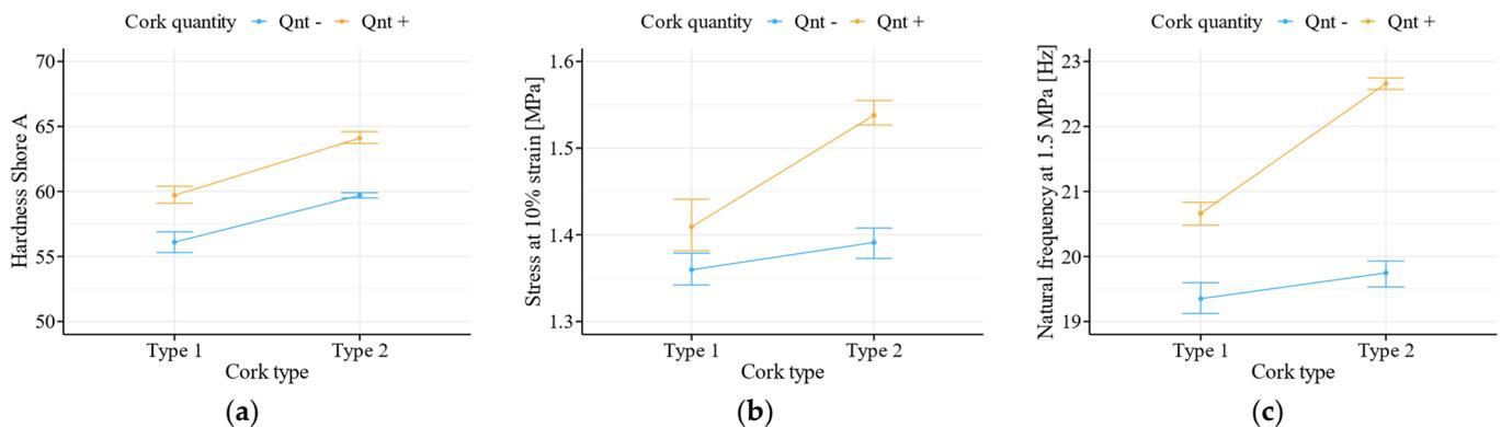
**Figure 4.** Results of cork analysis: interaction plots of: (a) Hardness Shore A; (b) Stress obtained at 10% compression strain; (c) Natural frequency when loaded at 1.5 MPa.
