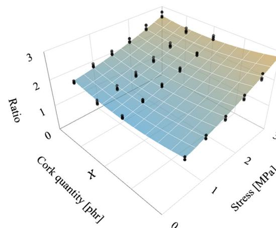
**Figure 10.** Experimental results and surface representing the regression model applied to predict the ratio between dynamic and apparent compression moduli.**Table 7.** Regression summary of dynamic behavior models.
