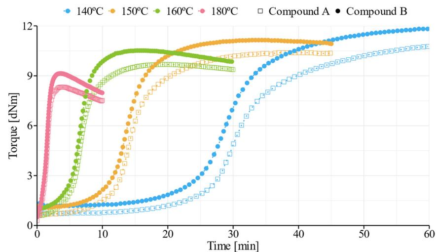
**Figure 7.** Rheometer curves obtained for compounds A and B at different vulcanization temperatures.
