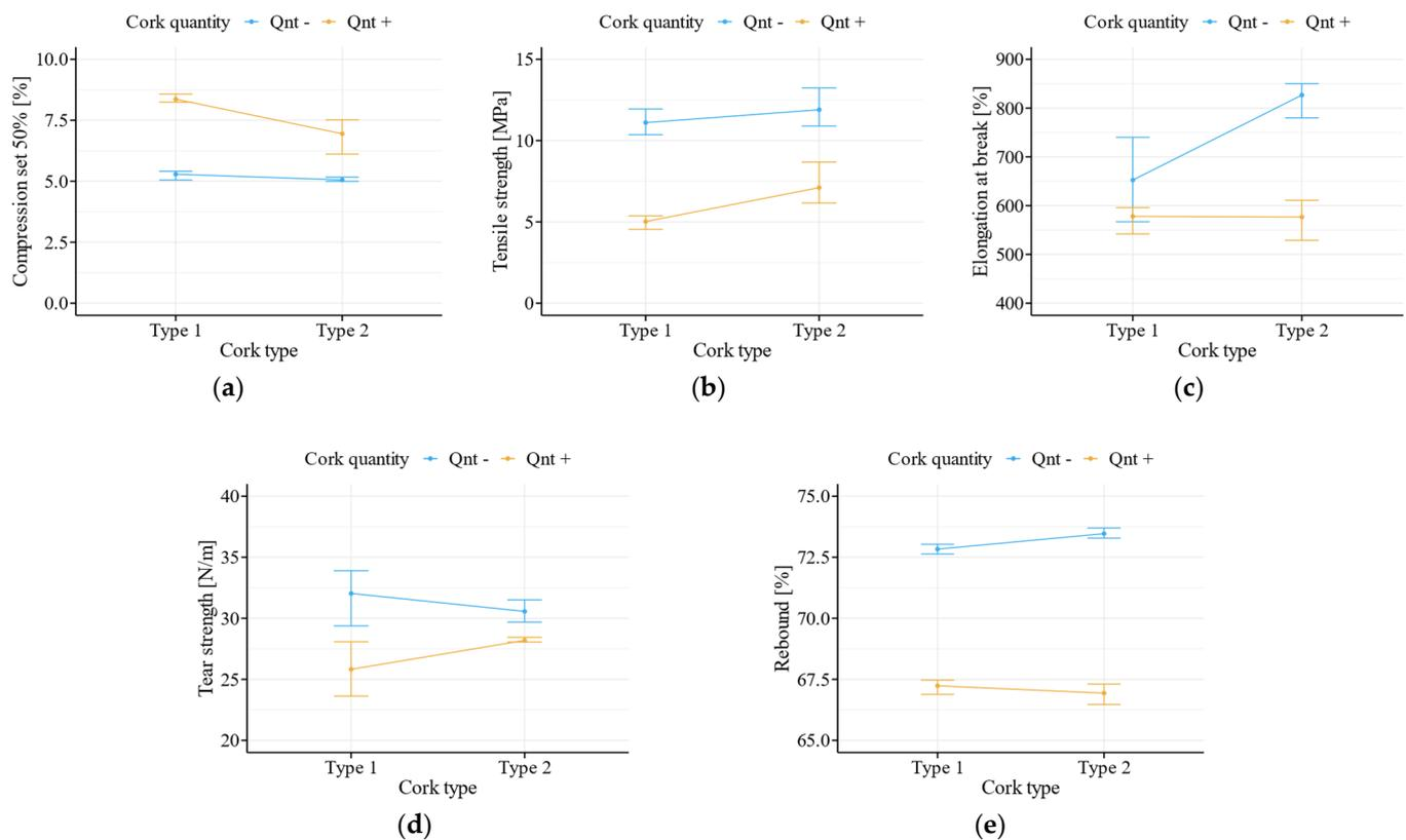
**Figure 5.** Results from cork analysis: interaction plots of: (a) Compression set; (b) Tensile strength; (c) Elongation at break; (d) Tear strength; (e) Rebound.
