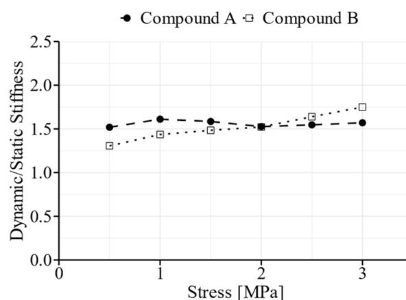
**Figure 1.** Effect of the addition of cork granules on the ratio between dynamic and static stiffness across different compression stress levels.
