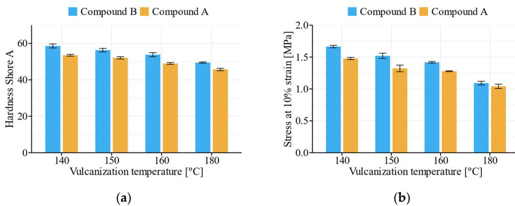
**Figure 6.** Results of vulcanization temperature analysis: (a) Hardness Shore A; (b) Static compression stress at 10% strain.
