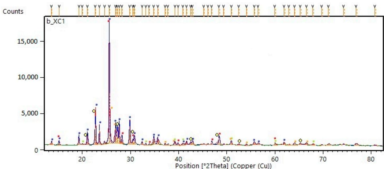
**Figure 3.** Diffraction pattern of a ceramic sample B20-1; phases: blue— $\text{KAlSi}_3\text{O}_8$ , red— $\text{LiAlSi}_2\text{O}_6$ , green— $\text{K}_{1.25}\text{Al}_{1.25}\text{Si}_{0.75}\text{O}_4$ , yellow— $\text{LiAlSi}_3\text{O}_8$ , orange— $\text{Al}_2\text{SiO}_5$ .
