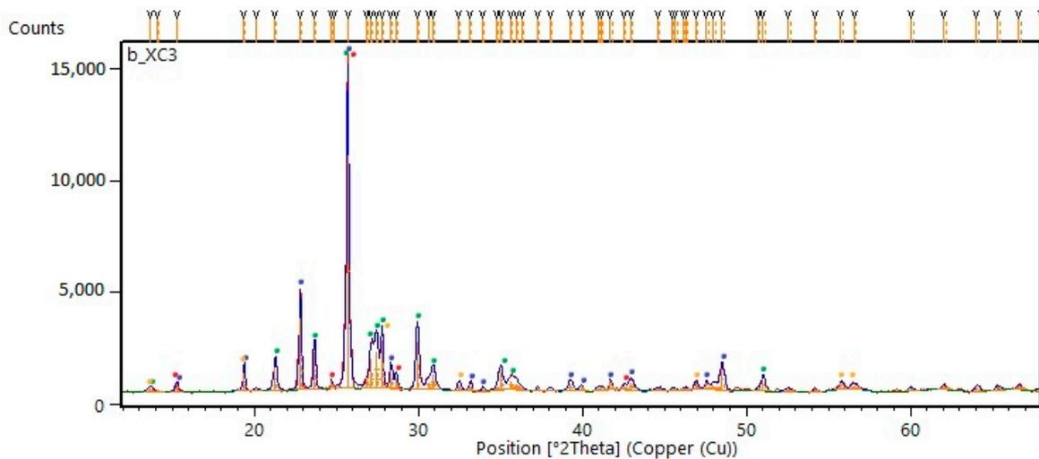
**Figure 5.** Diffraction pattern of a ceramic sample B20-3; phases: blue— $\text{LiAlSi}_3\text{O}_8$ , green— $\text{KAlSi}_3\text{O}_8$ , red— $\text{KAlSiO}_4$ , orange— $\text{SrAl}_2\text{Si}_2\text{O}_8$ ;  $\text{K}_{9.71}\text{Al}_{1.68}\text{Si}_{34.32}\text{O}_{72}$ .
