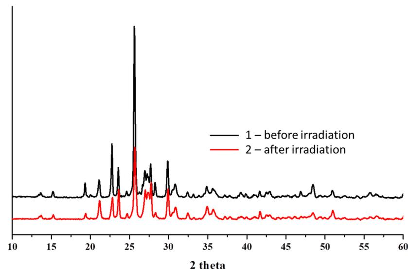
**Figure 11.** Comparison of the X-ray diffraction patterns of the sample B20-1 before irradiation (1) and after irradiation to the absorbed dose of  $10^9$  Gy (2).
