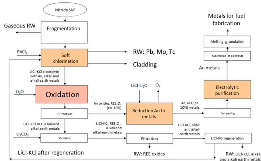
**Figure 1.** The technological optional scheme for pyrochemical processing of nitride SNF.
