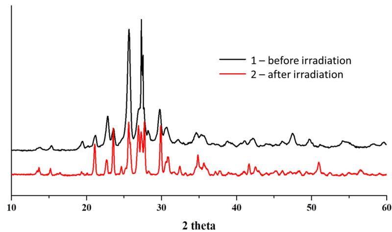
**Figure 12.** Comparison of the X-ray diffraction patterns of the sample B + mcrSi10 before irradiation (1) and after irradiation to the absorbed dose of  $10^9$  Gy (2).
