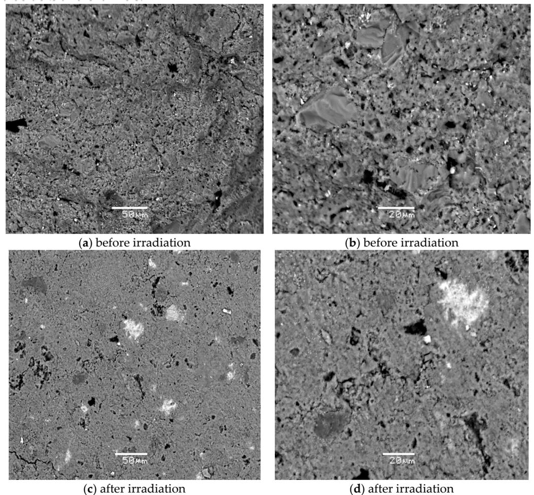
**Figure 13.** SEM images of the samples with composition B20-1 before and after irradiation by electrons to the absorbed dose of  $10^9$  Gy.
