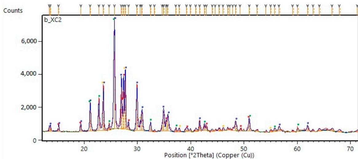
**Figure 4.** Diffraction pattern of a ceramic sample B20-2; phases: blue— $\text{KAlSi}_3\text{O}_8$ , green— $\text{LiAlSi}_3\text{O}_8$ , red— $\text{SrAl}_2\text{Si}_2\text{O}_8$ ,  $\text{Sr}_{46}\text{Al}_{92}\text{Si}_{100}\text{O}_{384}$ , orange— $\text{CsAlSi}_2\text{O}_6$ ;  $\text{Al}_2\text{SiO}_5$ .
