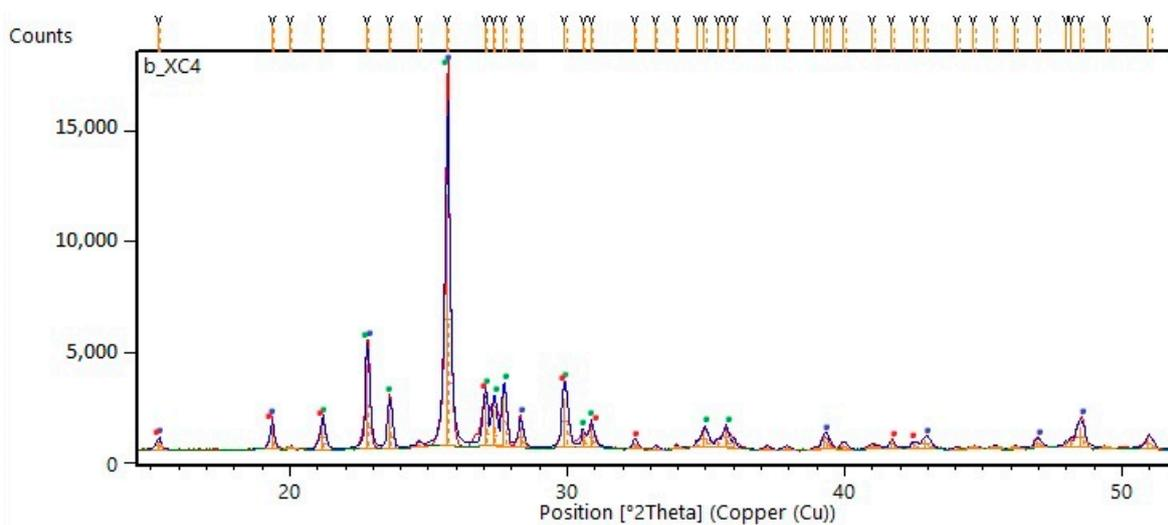
**Figure 6.** Diffraction pattern of a ceramic sample B20-4; phases: blue— $\text{LiAlSi}_3\text{O}_8$ , green— $\text{KAlSi}_3\text{O}_8$ , red— $\text{SrAl}_2\text{Si}_2\text{O}_8$ .
