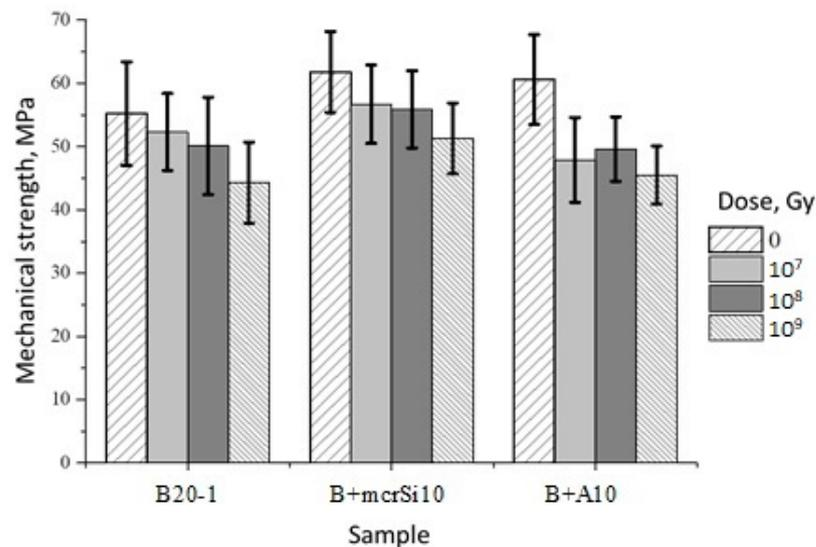
**Figure 10.** Dependence of the mechanical strength of samples on the dose of ionizing radiation.
