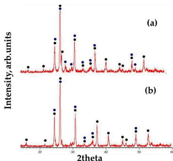
**Figure 8.** Diffraction patterns of auxiliary samples based on bentonite with an increased content of cesium chloride: black— $\text{CsAlSiO}_4$ ,  $\text{CsAlSi}_2\text{O}_6$ ; blue—other phases ( $\text{KAlSi}_3\text{O}_8$ ,  $\text{LiAl}(\text{SiO}_3)_2$ ,  $\text{Al}_2(\text{SiO}_4)\text{O}$ ). (a) 1/4 part of CIM is  $\text{CsCl}$ , 3/4 parts of CIM—eutectic  $\text{LiCl-KCl}$ ; (b) 1/2 part of CIM is  $\text{CsCl}$ , 1/2 part of CIM—eutectic  $\text{LiCl-KCl}$ .
