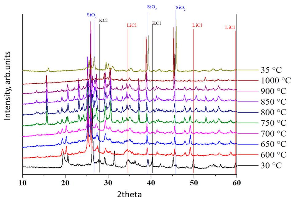
**Figure 7.** Diffraction patterns of a sample based on bentonite clay with the inclusion of 30 wt.% of simulated spent eutectic LiCl–KCl obtained at different temperatures.
