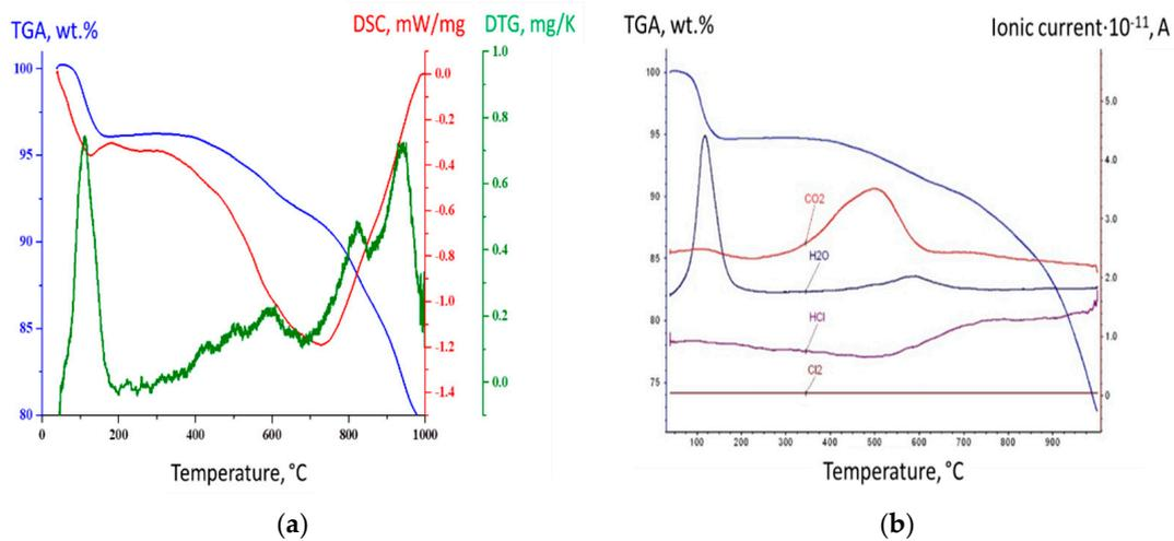
**Figure 2.** (a) TGA and DSC curves for a sample B20-0; (b) TGA curves together with the composition of the released gases according to mass spectrometry data.
