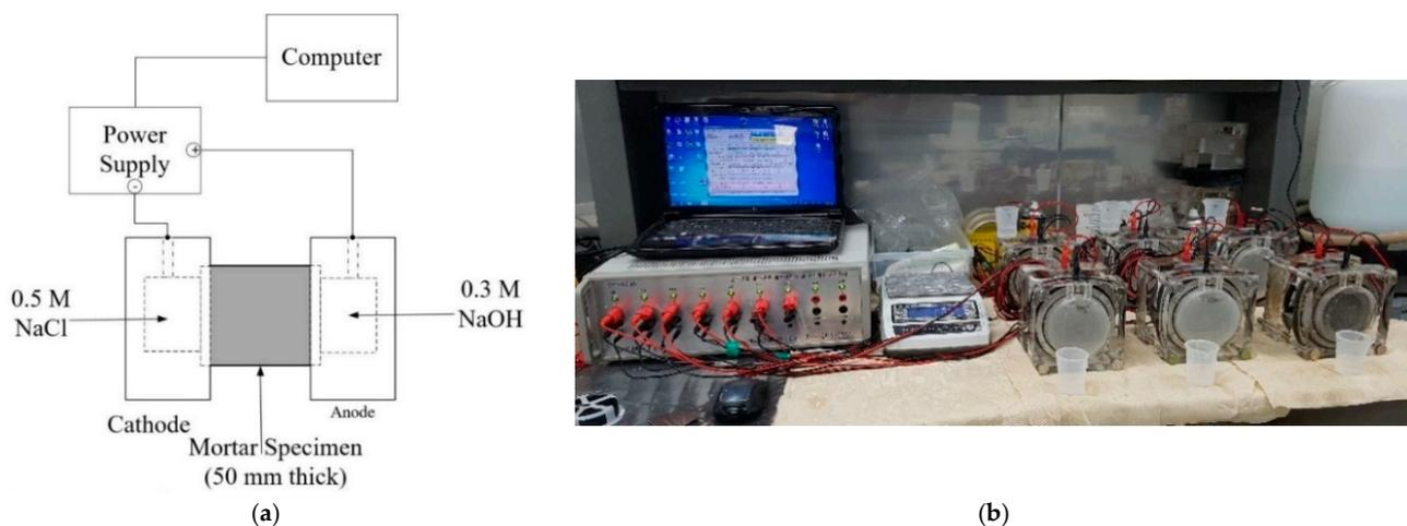
**Figure 2.** Test setup for chloride migration test; (a) schematic diagram [36]; (b) pictorial view of the test setup.
