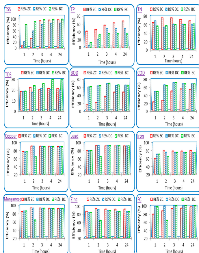
Figure 4. Percentages of removal efficiency (RE%) for TSS, TN, TP, TDS, BOD, COD, copper, lead, iron, manganese, zinc and FC removed from wastewater by zeolite (ZC), diatomite (DC), and bentonite (BC) columns.
