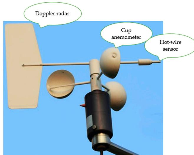
**Figure 4.** Cup and hot-wire, hybrid anemometer, Reprinted from Francisca et al. [40] with permission under the terms of the Creative Commons Attribution License. <http://creativecommons.org/licenses/by/4.0>.
