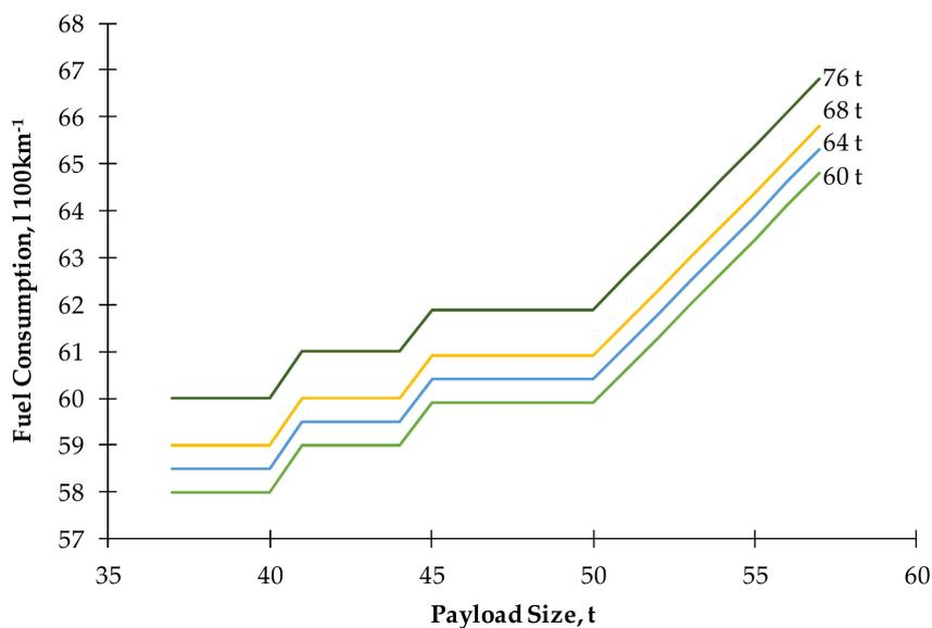
**Figure 7.** Fuel consumption of the vehicle combinations to varying payload sizes.
