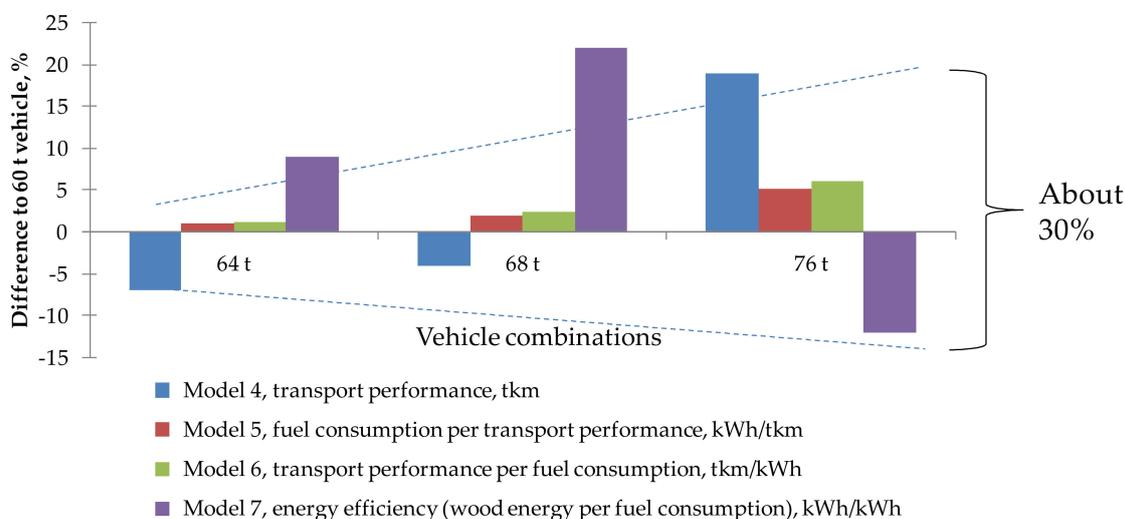
**Figure 9.** Energy efficiency differences between 64, 68, and 76 t vehicle combinations in comparison with the 60 t vehicle combination using four different energy efficiency measurements in the same wood supply region.
