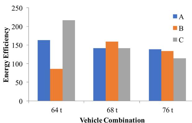
**Figure 10.** Energy efficiency comparison between the vehicle combinations of the STSs in three wood supply regions (A, B, C) of the eastern study area: Energy efficiency is calculated as the energy content of 100% renewable wood (kWh) per energy content of fuel consumption (kWh) of laden vehicles (Model 7). Energy efficiency is compared to carbon neutral level (0).
