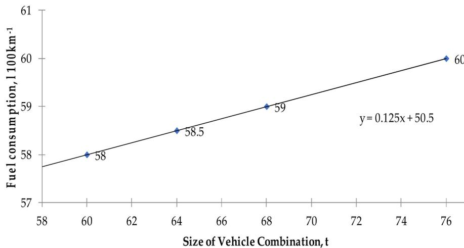
**Figure 6.** The average fuel consumption of a vehicle combination with a payload size of 37 t.
