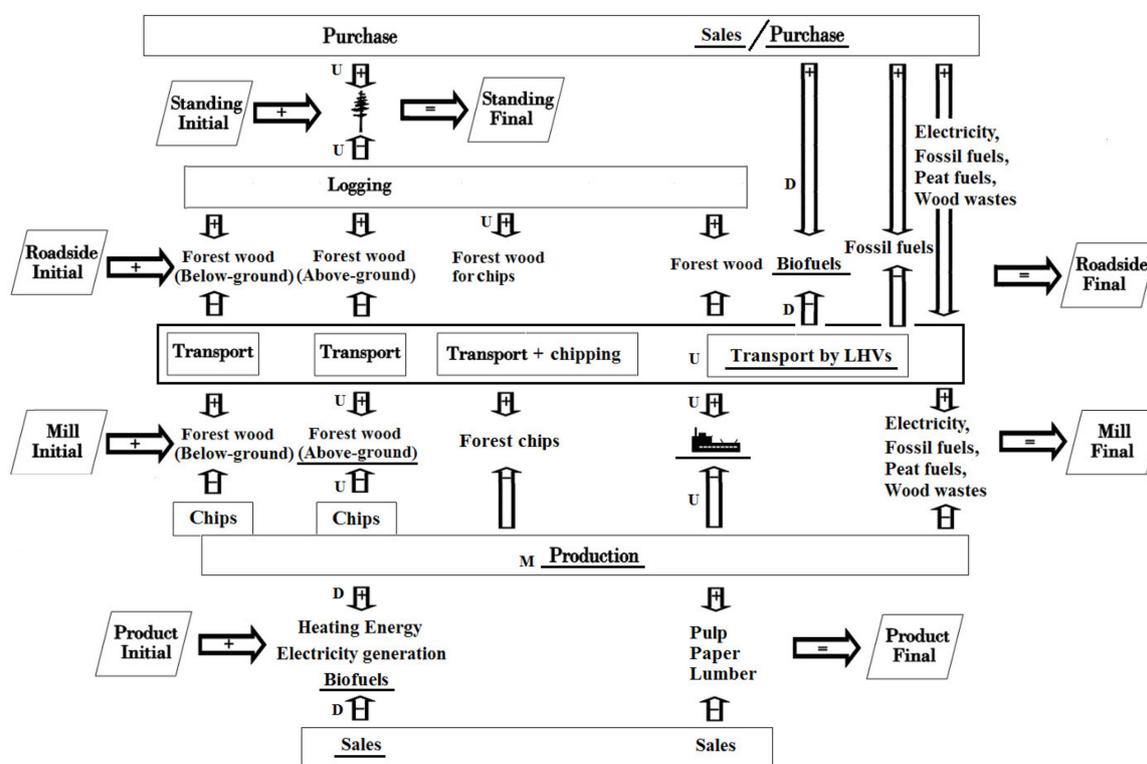
**Figure 2.** Dynamics of a supply system's material, energy, and monetary flows. Overview of inventories (states), operations (stages), and a sustainable cycle of advanced biofuels for the engines of larger and heavier vehicles for road freight transportation is underlined in the supply system. U = upstream; M = midstream; D = downstream.
