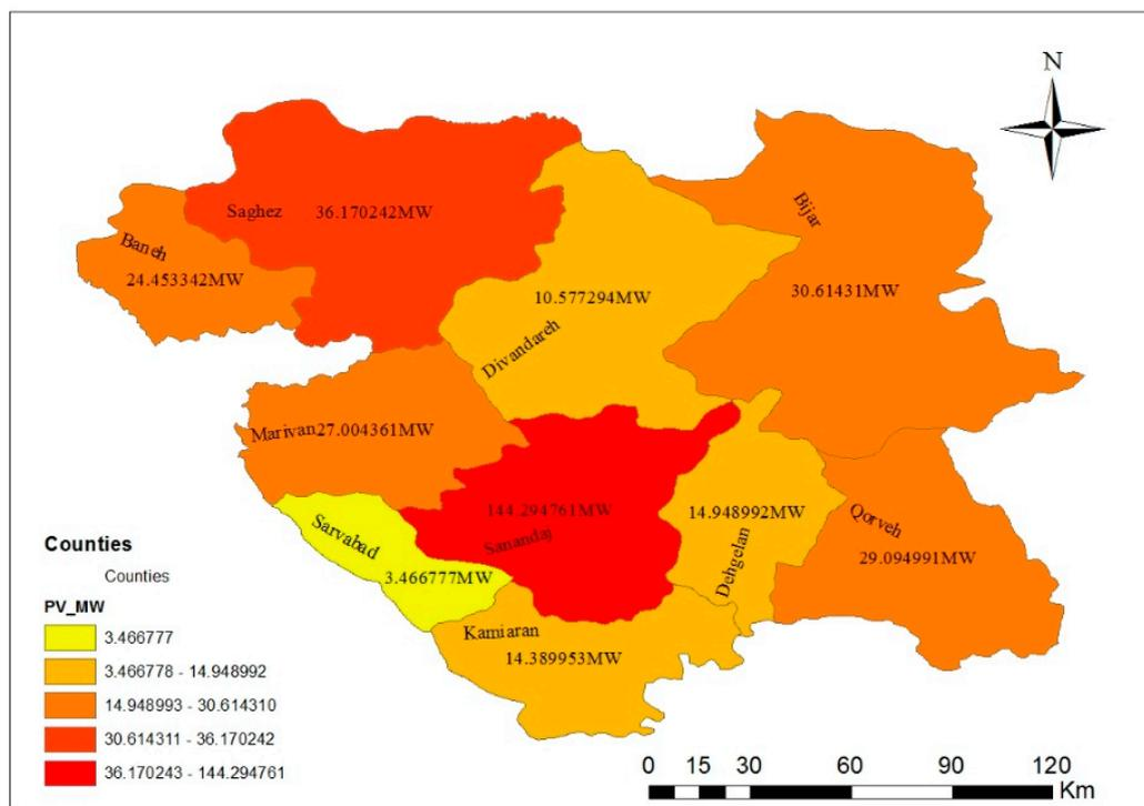
Figure 11. Potential of domestic photovoltaic in Kurdistan.
