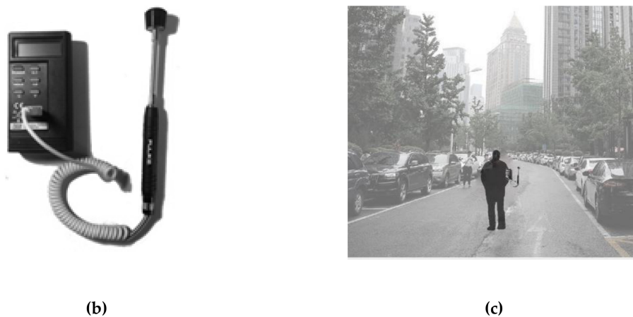
Figure 4. (a) Range and form of Xijiekou Centralized Zone (XCZ) and distribution of measurement points (with numbered-round circle); (b) TES-1310 portable electronic thermodetectors; (c) scene of measurement.
