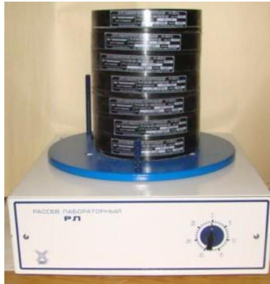
**Figure 11.** Laboratory plansifter RL brand with a set of sieves for determining the granulometric composition of the forage.
