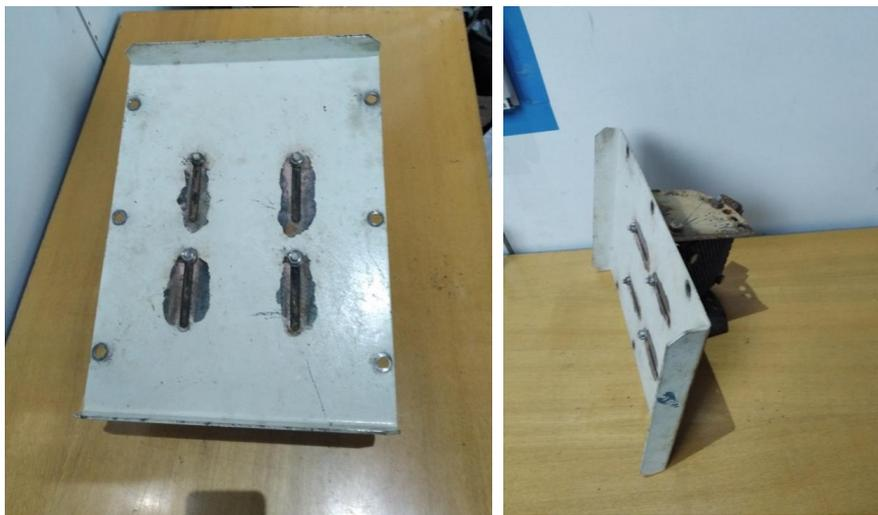
**Figure 6.** Cover with slots for adjusting the clearance S between the grid-work (plate) and the nozzle.
