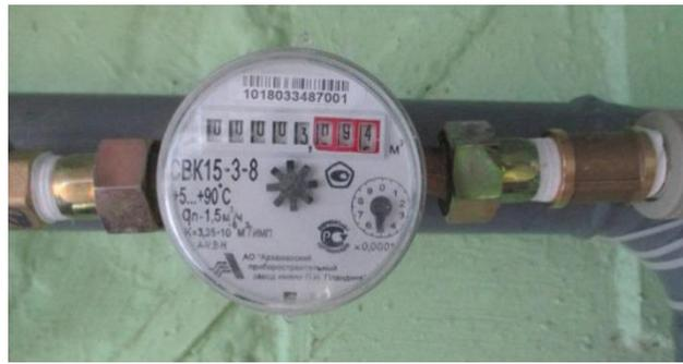
**Figure 2.** Water meter SVK 15-3-8 used for recording the amount of water poured into the tank of the measuring station.
