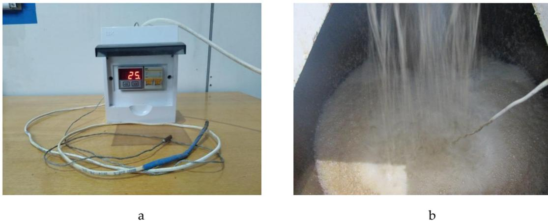
**Figure 10.** Temperature controller TL-11-250 with a temperature sensor TST81 (a) and recording the temperature of the forage from grain (b).
