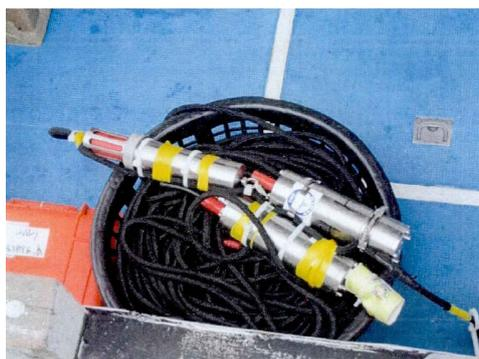
**Figure 8.** The H<sub>2</sub>S microelectrode integrated in a multi-parameter chemical sensor [69].
