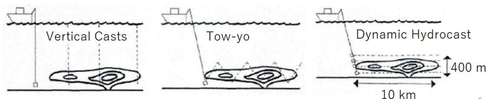
**Figure 2.** Vessels search HT plume using integrated multi-sensors [52]. The chance of encountering the HT plume can be enlarged by adjusting the depth of the towed sensors during the survey, or by using a vertical array of sensors.
