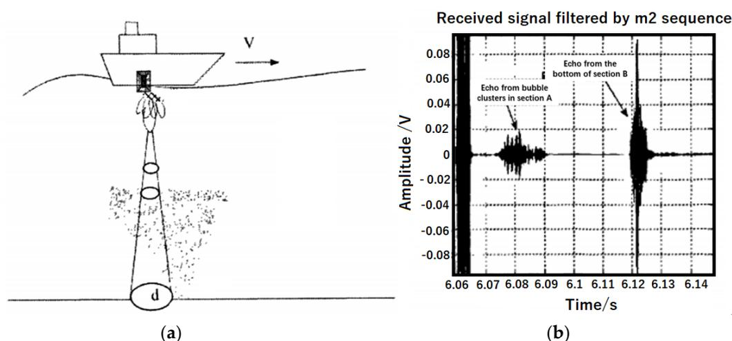
**Figure 5.** Acoustic detection of bubble clusters associated with HT vents. (a) The sketch map of detecting bubble clusters; (b) the reflection signal received after filtering. The smaller peak indicates the position of bubble clusters. The larger peak indicates the depth of the lake [63].
