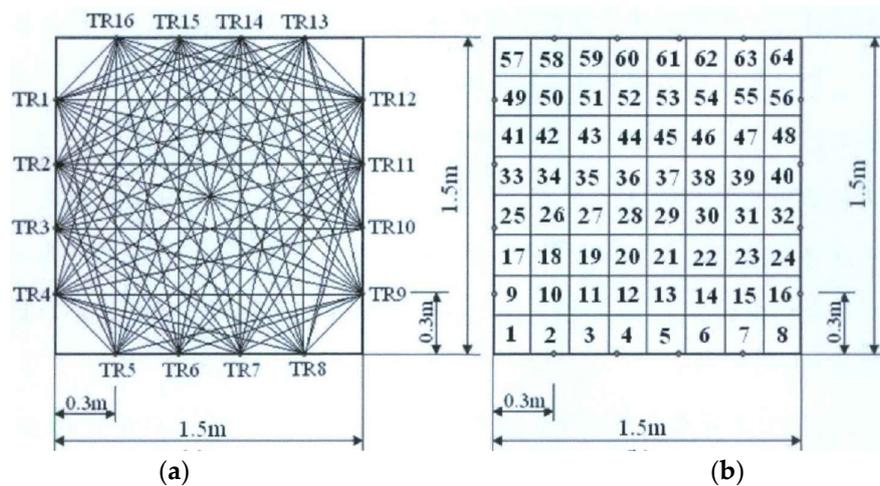
**Figure 11.** The reconstruction of 2D temperature field using acoustic tomography. (a) The distribution of hydrophones and corresponding acoustic paths on the measuring plane; (b) the meshed plane for the reconstruction of 2D temperature distribution using the total least-squares method [72].
