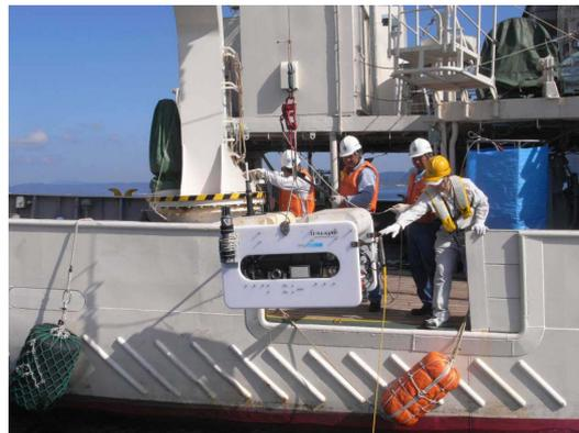
**Figure 3.** TUNA-SAND and its survey in Kagoshima Bay, Japan. The ROV was released from the vessel and surveyed at a depth of approximately 200 m, searching for evidence of undiscovered HT vents [56].
