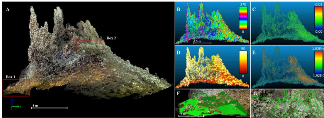
**Figure 9.** South side of reconstructed 3D textured dense point cloud and derived terrain variables [74]. (B) shows the aspect of chimney; colors on (C) show the different roughness; (D) shows the inclination of slope, with a maximum value of 90 degrees. (E) shows the Gaussian surface curvature. (F,G) are detailed views of box 1 and box 2 in figure (A), respectively.
