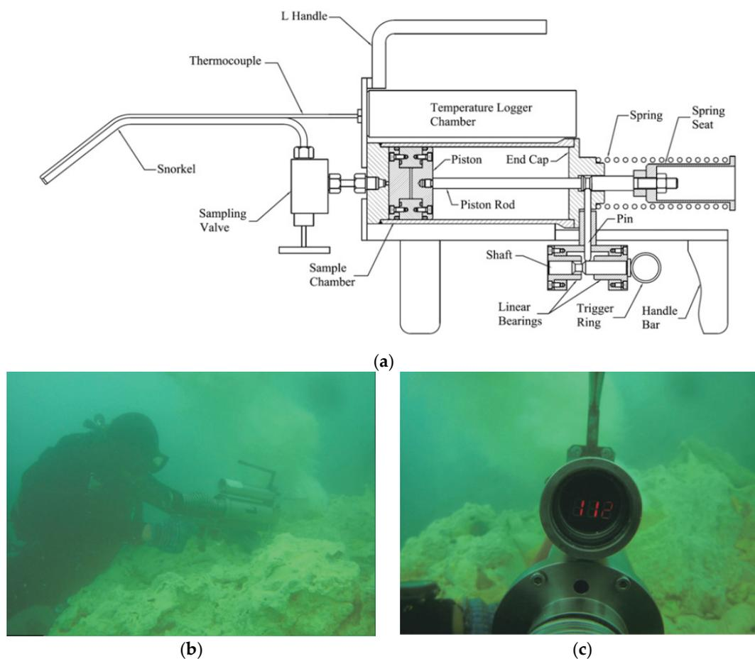
**Figure 13.** The handheld sampler developed for SHT sampling. (a) The structure diagram of the sampler; (b) collecting organic samples from the orifice of a yellow vent in the Kueishan Tao vent field; (c) the real-time measurement while sampling [82].
