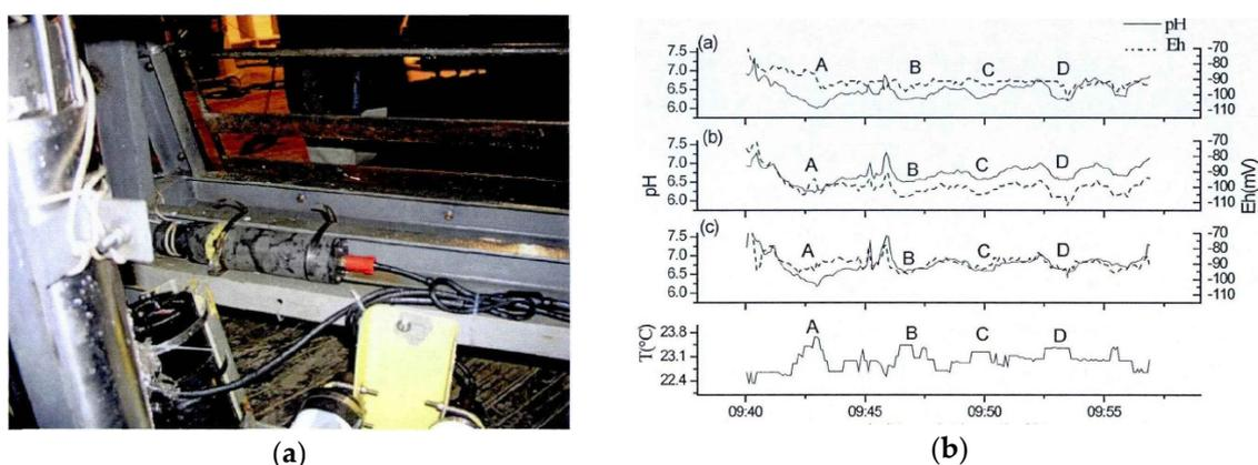
**Figure 7.** The IrO<sub>2</sub> electrode applied in SHT studies in Kueishan Tao HT vent areas. (a) The integrated sensors; (b) pH and temperature measured in the HT plume of a yellow vent. The three pH curves refer to the pH measured at depths of 3, 5 and 7 m, respectively. The letters A, B, C and D mark the variation cycle of the temperature. When the temperature rises, the values of pH and Eh drop, indicating that the area is under the influence of HT fluids [68].
