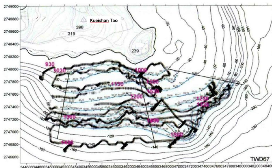
**Figure 4.** The navigation track of the survey south-east of Kueishan Island [57]. The sensor chain containing 6 sensors was released and towed during the survey. Data suggests the existence of undiscovered SHT vents in the surveying area.
