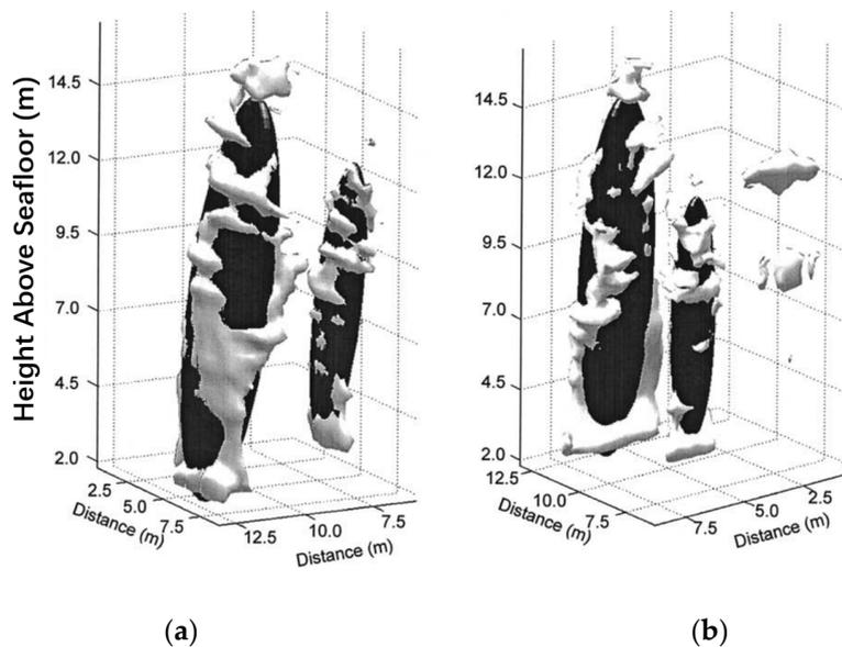
**Figure 10.** The front (a) and back (b) views of the reconstructed 3D image of two adjacent HT plumes [76]. The grey part in the figure shows the patterns of the HT plumes. The black part is the ellipsoids fitted to show the roughness of a plume.
