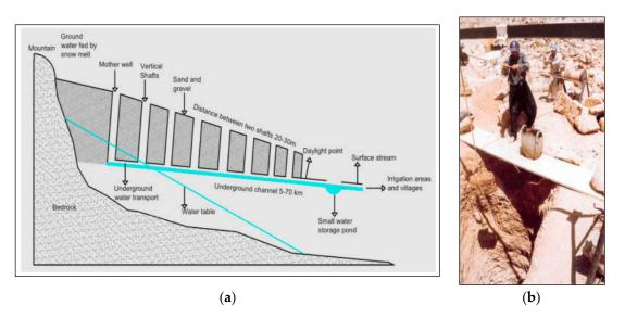
**Figure 1.** Qanat system: (**a**) sketch of a qanat transporting water from upland to lowland areas [19]; (**b**) cleaning of a 1500-year-old qanat in Syria [20].
