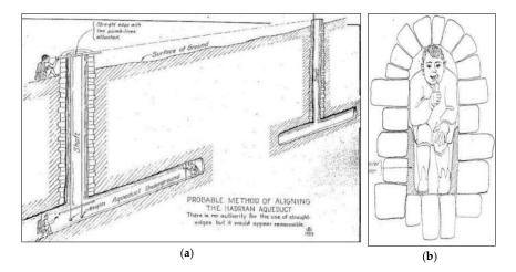
**Figure 13.** Hadrian aqueduct of Athens: (**a**) method of tunnel alignment; (**b**) cross section of a narrow sector of the tunnel, at the limit of the working possibility [49].
