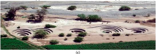
**Figure 19.** System of *puquios* (qanat-like aqueduct with spiraling shaft) at Cantalloc (Southern Peru, Nazca culture, ca 2nd–7th century AD): (a) aerial view of the central part of the system; (b) ground level photo of a well 8–10 m deep, with scale [64]; (c) the first five (right-to-left) mother wells of the line, fed by the water table of the paralleling dry riverbed (view to N) [62].
