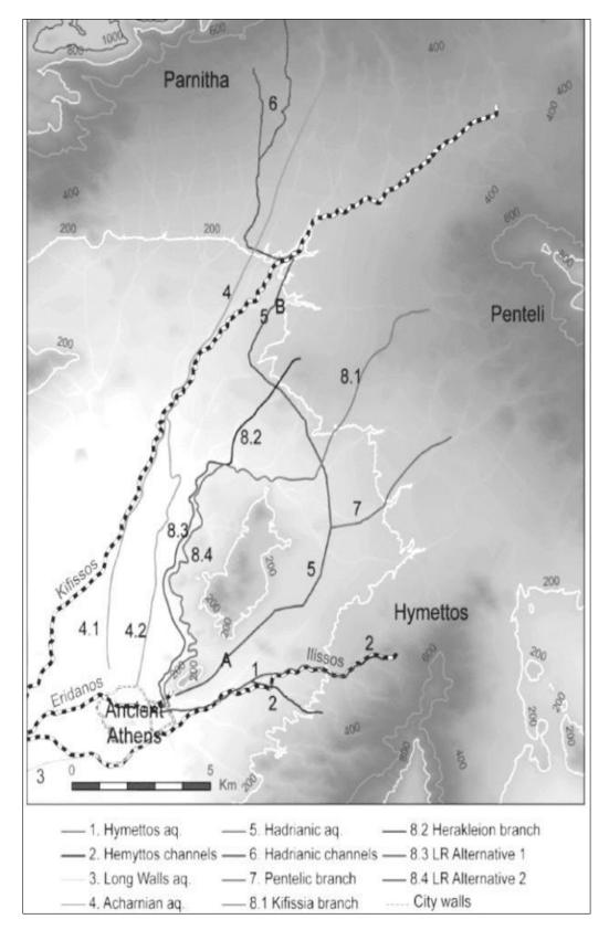
**Figure 8.** Probable routes of the ancient aqueducts in the basin of Athens [33] with the *Peisitrateian* marked with numbers 1 and 2.
