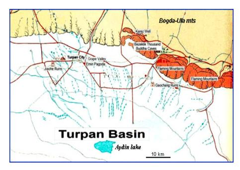
**Figure 20.** Karez lines (in blue) of the Turpan basin, distributed along the southern slopes of the Bogda-Ula mountains. In the last 50 years, the number of karez active systems decreased from 1000 to 480 [70].
