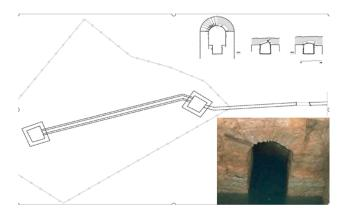
**Figure 22.** The aqueduct of Pylos at the Chandrinos spring. Top: the mid-19th c. square wells connected with an arched gallery under a protective coverage of concrete. Right bottom: the opening of the arched gallery [71].
