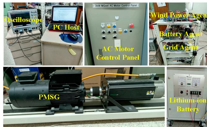
Figure 15. Configuration of the experimental DCMG system.
