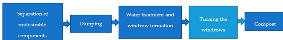
Figure 3. Process of composting of municipal solid waste management.
