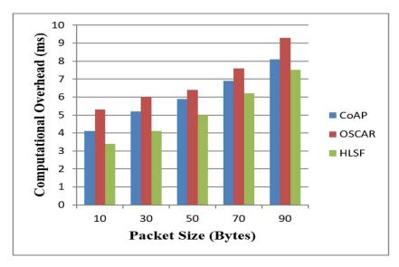
Figure 10. Computational overhead for CoAP, OSCAR, and HLSF.
