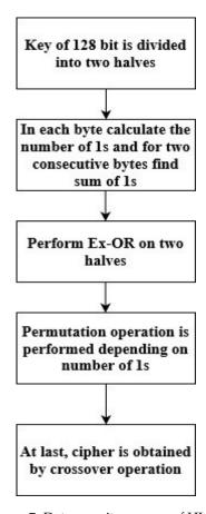
Figure 7. Data security process of HLSF.
