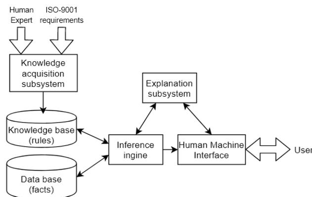
Figure 5. System architecture.
