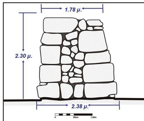
**Figure 4.** A schematic design of the dyke in Kopais [14].
