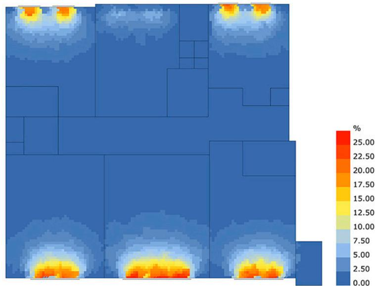
**Figure 13.** Grid-based daylight factor (DF) analysis from 0% (dark blue) to 25% (dark red).
