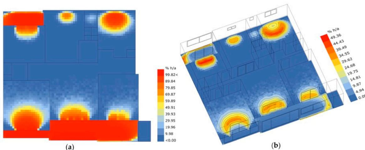
**Figure 9.** (a) Annual Daylight Autonomy (DA) map and (b) Useful Daylight Illuminance (UDI) analyses for the reference apartment unit.
