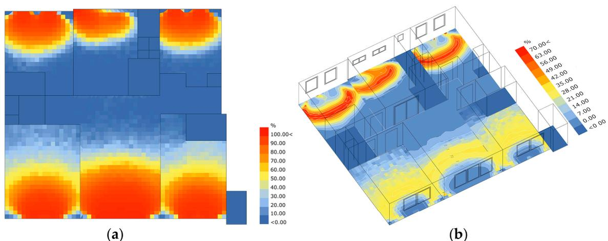
**Figure 14.** Reference apartment annual grid-based daylight autonomy (DA) and useful daylight illuminance (UDI) analyses; (a) DA analysis of the apartment unit's floor plan from 0% (dark blue) to 100% (dark red); (b) UDI analysis of the isometric apartment floor plan layout from 0% (dark blue) to 70% (dark red).
