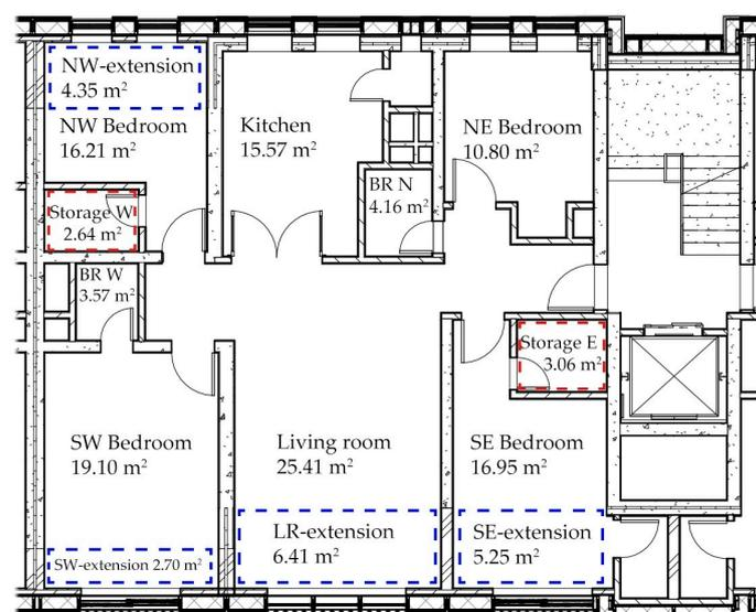
**Figure 10.** Virtual BIM model of the renovated apartment showing the exterior enhanced building envelope system and the reconfiguration of the interior spaces, with indication of the cumulative floor space of each room and extension/storage areas.
