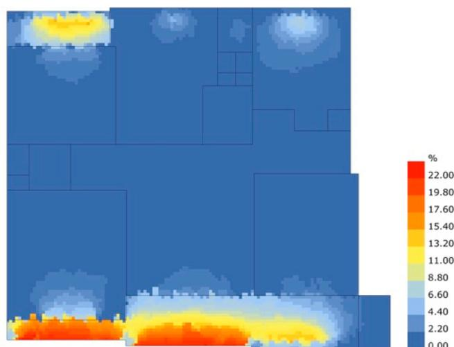
**Figure 8.** Daylight factor (DF) ground floor map for the reference apartment unit with illustration of the DF in the majority of 0% (dark blue) to 22% (dark red).
