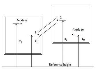
Figure 3. Concept map of the airflow network model.
