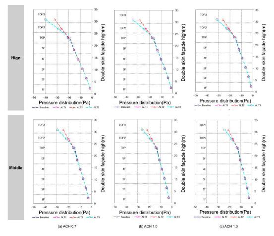
Figure 16. Pressure distribution by ACH with high and middle levels of solar irradiance.
