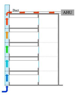
Figure 10. Concept of the simulation model for outdoor air (OA)-based air conditioning in winter.
