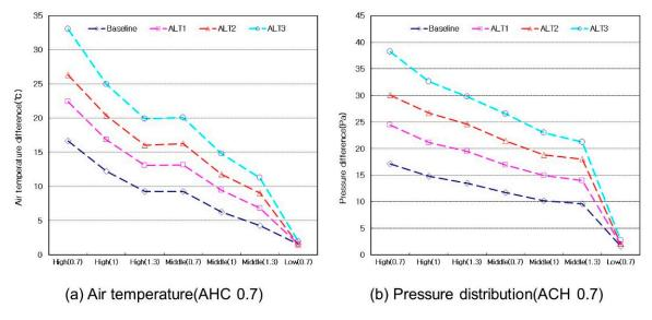
Figure 18. Air temperature and pressure difference by ACH.
