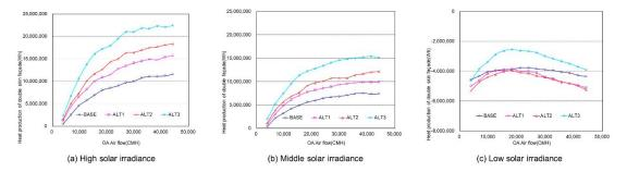
Figure 13. Heat gain of the double skin facade by ALT and solar irradiance.
