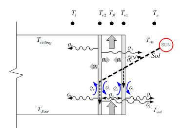
Figure 2. Overview of the basic theory of heat transfer in double-skin facades.
