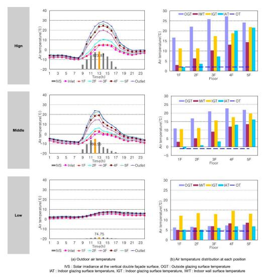
Figure 8. Air temperature at double skin façade by solar irradiance in winter.
