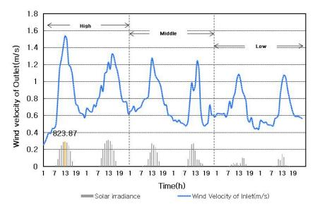
Figure 9. Wind velocity distribution of the Outlet in winter.
