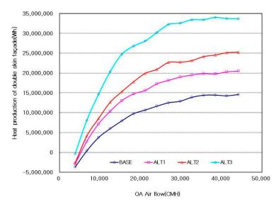
Figure 14. Heat production of the double skin facade by the OA airflow of the ALT.
