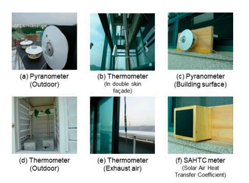
Figure 4. Photographs of Measuring Devices.
