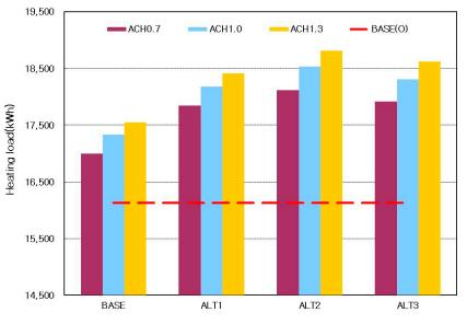
Figure 20. Heating load distribution by ACH of ALTs.
