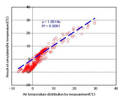
Figure 11. Comparison of air temperature between measurement and simulation results.
