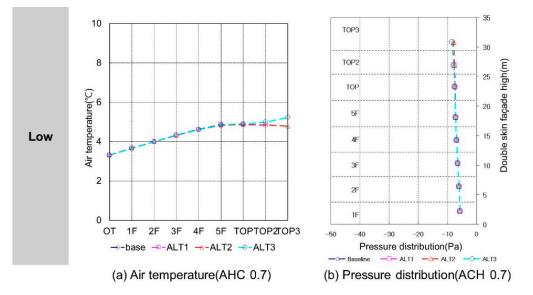
Figure 17. Air temperature and pressure distribution with low solar irradiance.
