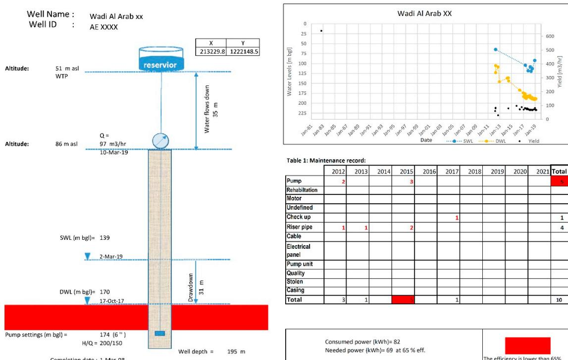
Figure 7. Operational decision support tool for wellfield management.
