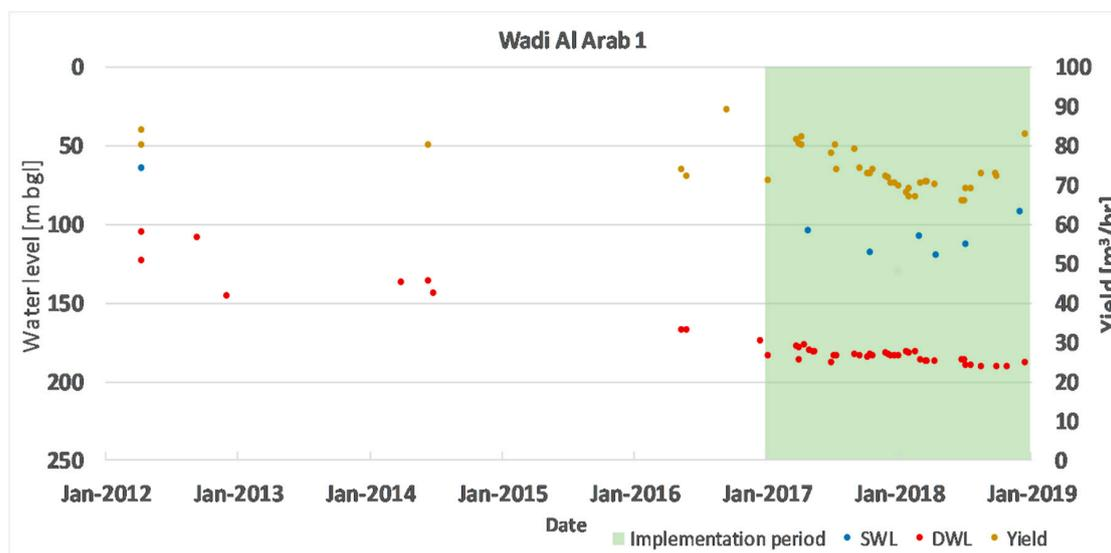
Figure 16. Improvement of field measurements (SWL, DWL and yield) before and during the implementation period of the tools, using WA-1 well as an example.
