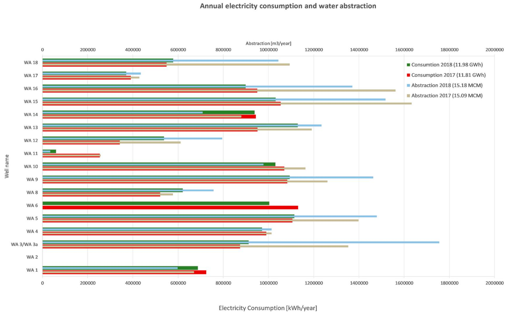
**Figure 12.** Electricity consumption and production in the wells of Wadi Al Arab (WA) wellfield in 2017 (no abstraction and electricity consumption as WA2. WA3 and WA3a had one electricity meter, no abstraction data was found for WA 6 as it doesn't pump water to the WA pumping station).
