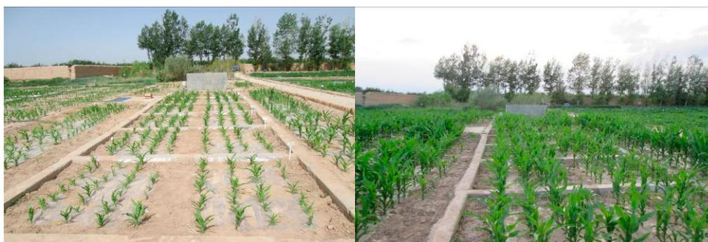
Figure 2. Non-weighing lysimeters used in the experiments.
