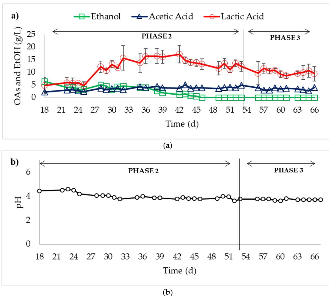
**Figure 2.** Process monitoring during phases 2 and 3, with inoculum addition: (a) organic acids (OAs) and ethanol (EtOH); (b) pH.
