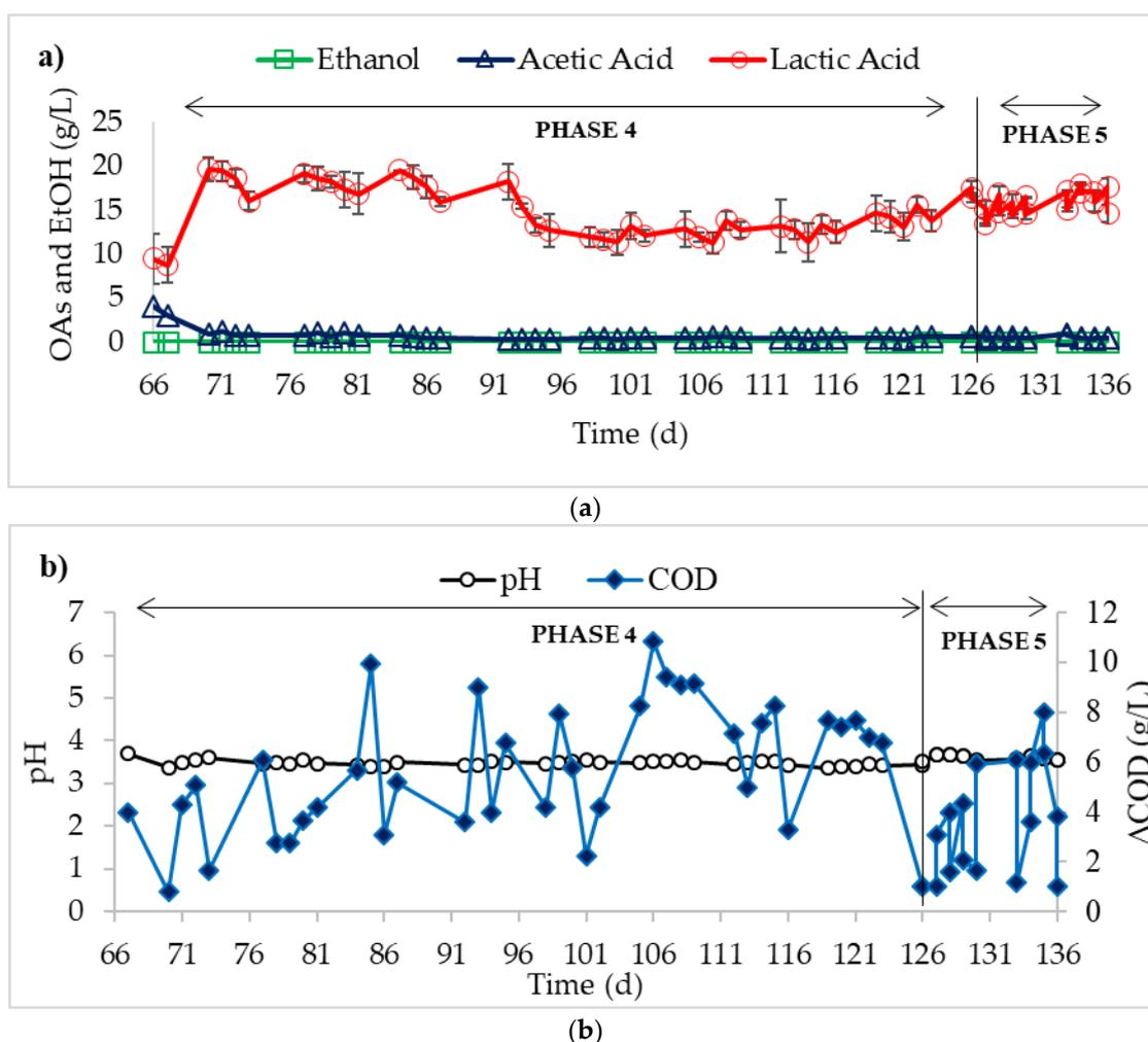
**Figure 3.** Process monitoring during phases 4 and 5, without inoculum addition: (a) OAs and EtOH; (b) pH (round indicators) and  $\Delta$ chemical oxygen demand (COD) (square indicators).
