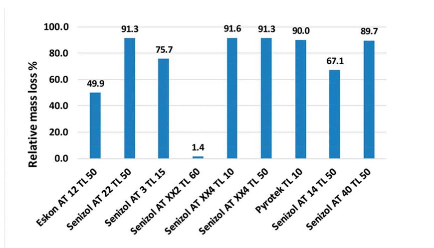
Figure 5. Mass loss of all tested materials.
