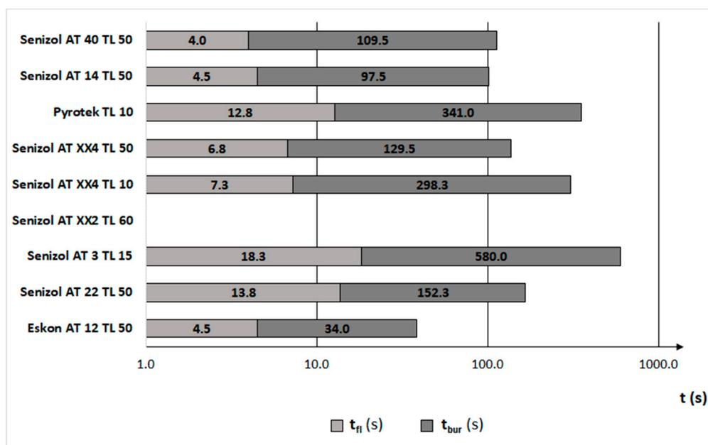
Figure 6. Flash time  $t_{fl}$  and flame burning time  $t_{bur}$  of tested products.
