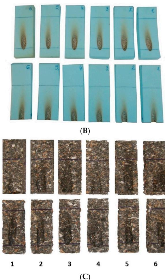
**Figure 8.** Polystyrene (A), polyurethane foam (B) and Senizol AT XX2 TL 60 (C) after ignitability test.
