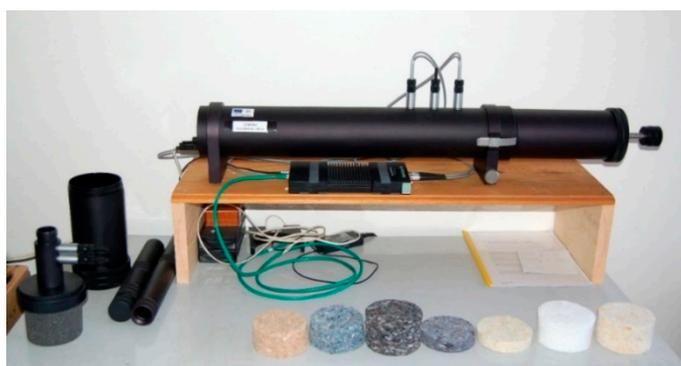
**Figure 4.** Kundt impedance tube Type 4206 and STERED<sup>®</sup> samples.
