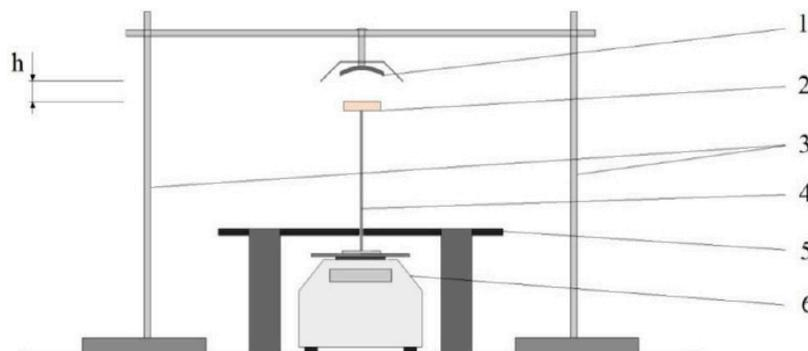
**Figure 3.** Scheme of test equipment [19] 1—ceramic infrared heater, 2—test sample, 3—metal frame, 4—sample holder, 5—scales protection, 6—analytical scales.
