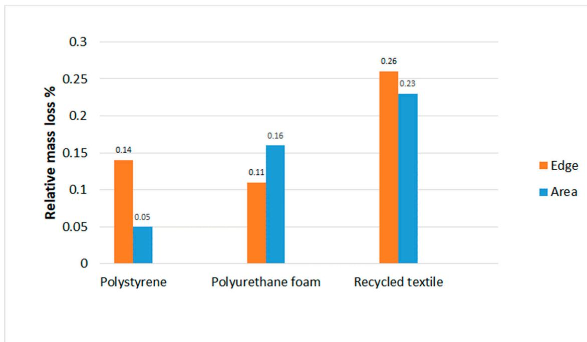
Figure 7. Evaluation of relative mass loss during the ignitability test.
