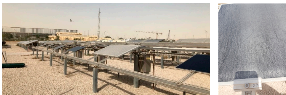
Figure 1. Five PV panels being tested in solar testing facility and a dusty PV panel surface before cleaning.
