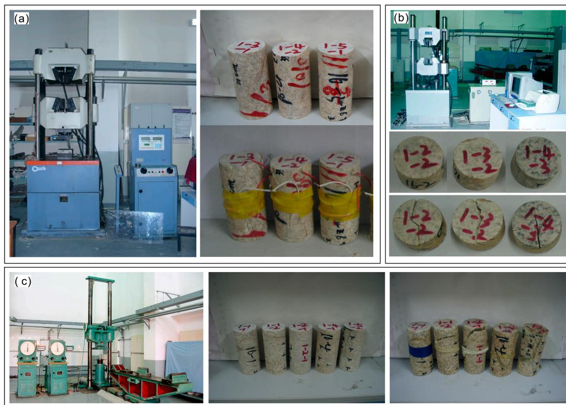
**Figure 7.** Laboratory test of the surrounding rock. (a) Uniaxial compression test, (b) Brazilian disc test, (c) triaxial compression test.
