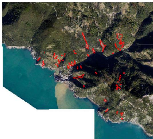
**Figure 6.** The same area of Figure 1 on November 2011 after the rainfall event of 25 October 2011. The landslides are emphasized in red. It's clear how woodland substituted agriculture in the last 40 years.
