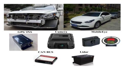
Figure 3. Experimental vehicle and equipment.
