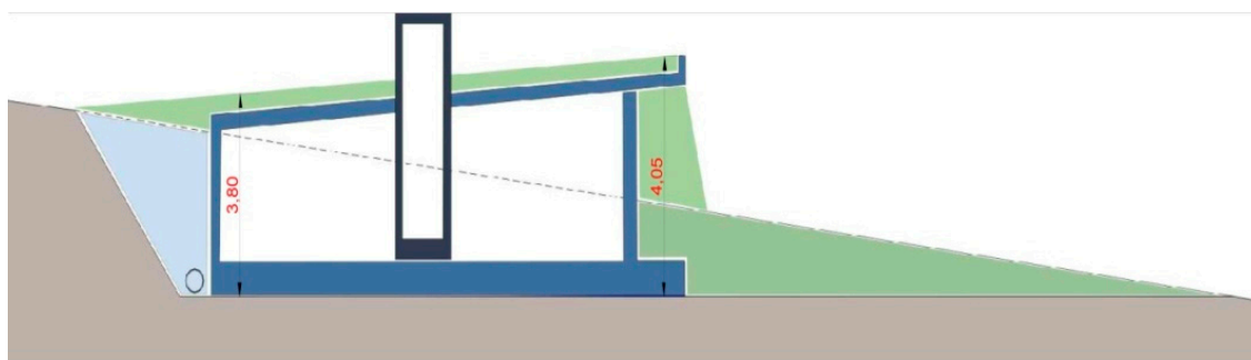
Figure 12. Cross section of Dobraca house with the soil cover measure (Source: authors).
