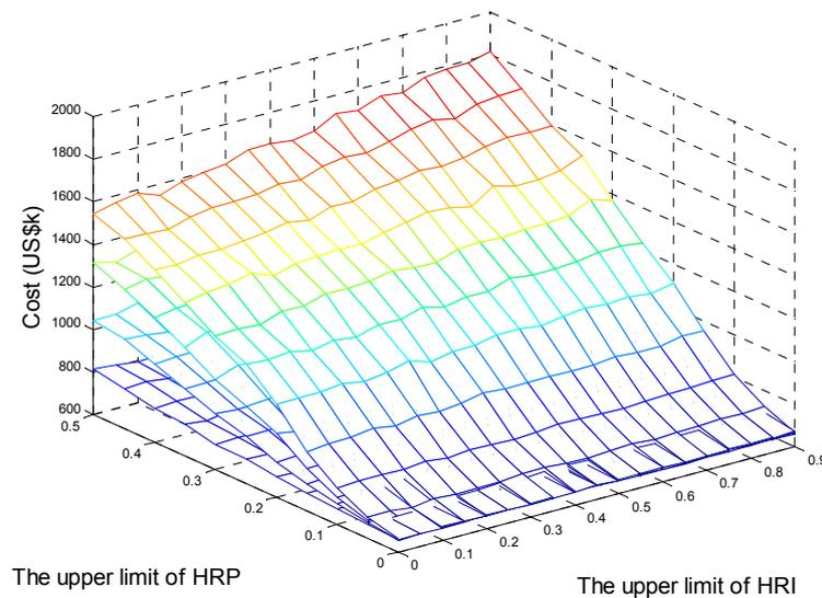
Figure 10. Relationships between rework parameters and cost.
