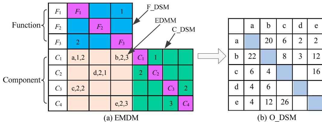
Figure 3. Organization design structure matrix (O\_DSM) derivation process.
