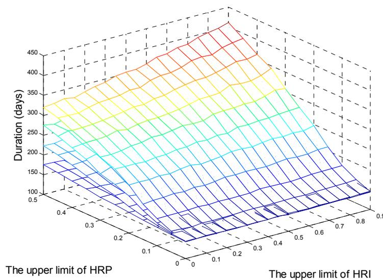
Figure 9. Relationships between rework parameters and duration.
