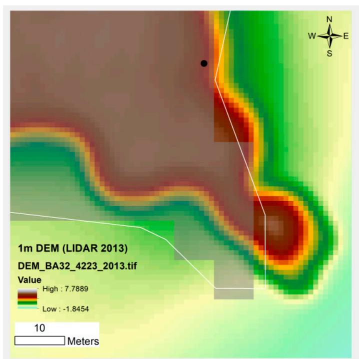
**Figure 20.** Example of highest current resolution digital elevation model. This site location is shown relative to 1 m resolution DEM (LiDAR) compared with 8 m resolution DEM. On 25 m resolution DEM, this site is estimated to be at sea level.
