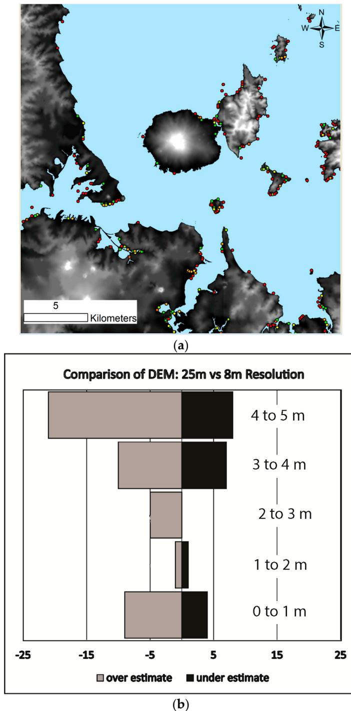
**Figure 19.** Sea level rise modeling with higher resolution digital elevation model (8 m resolution DEM). Map of detailed study area (a) shows sites at risk. If we assume that the 8 m resolution DEM provides a better estimate of the position of sites relative to current sea level, than it would appear the 25 m DEM performed well (b).
