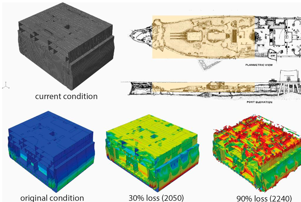
Figure 14. Computer model of the USS Arizona with projected decay of structure. Source: [62].
