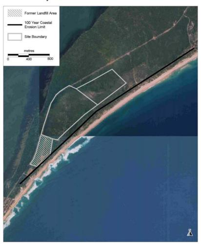
Figure 3. Estimated 100 year coastal erosion limit and location of former landfill.
