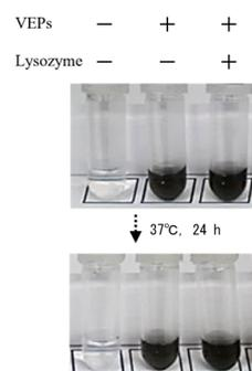
**Figure 6. Form of VEPs in lysozyme solution.** To clarify the solubility of VEPs with enzymatic treatment, VEPs were suspended in 100 μg/mL human lysozyme (Sigma-Aldrich, Tokyo, Japan) solution in 10 mM citrate buffer (pH 5.0) and incubated at 37 °C. After 24 h, the VEPs were resuspended by vortexing and photographed and imaged with a DSLR camera.
