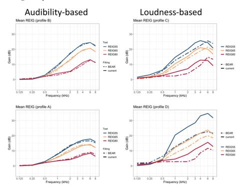
**Figure 4.** Mean real-ear insertion gains measured as part of the clinical study. Each panel shows data for one profile. Measurements made on participants fitted with the "current" strategy are shown with solid lines, while those made with the "BEAR" strategy are shown with dashed lines. The blue, yellow, and red lines represent input levels of 55, 65, and 80 dB SPL, respectively.
