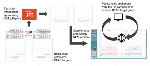
Figure 2. Illustration of the BEAR fitting tool and procedure developed for the clinical study.
