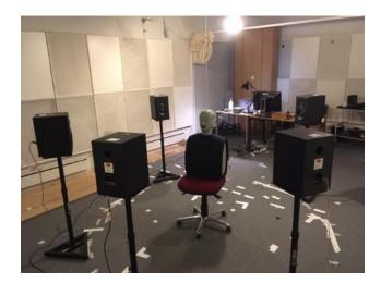
Figure 3. Picture of the test setup used for performing the SNR improvement measurements.
