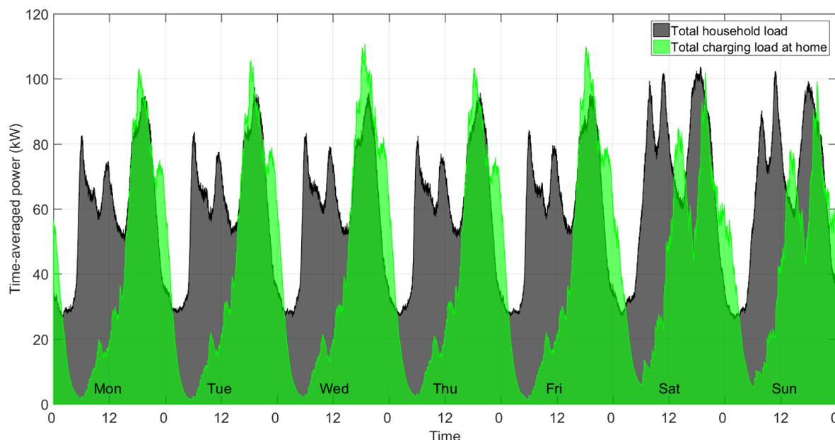
Figure 7: Averaged charging profile of stochastic generated EV loads (one week, 216 electric vehicles, charging power: 3.7 kW single phase, location "Home")
