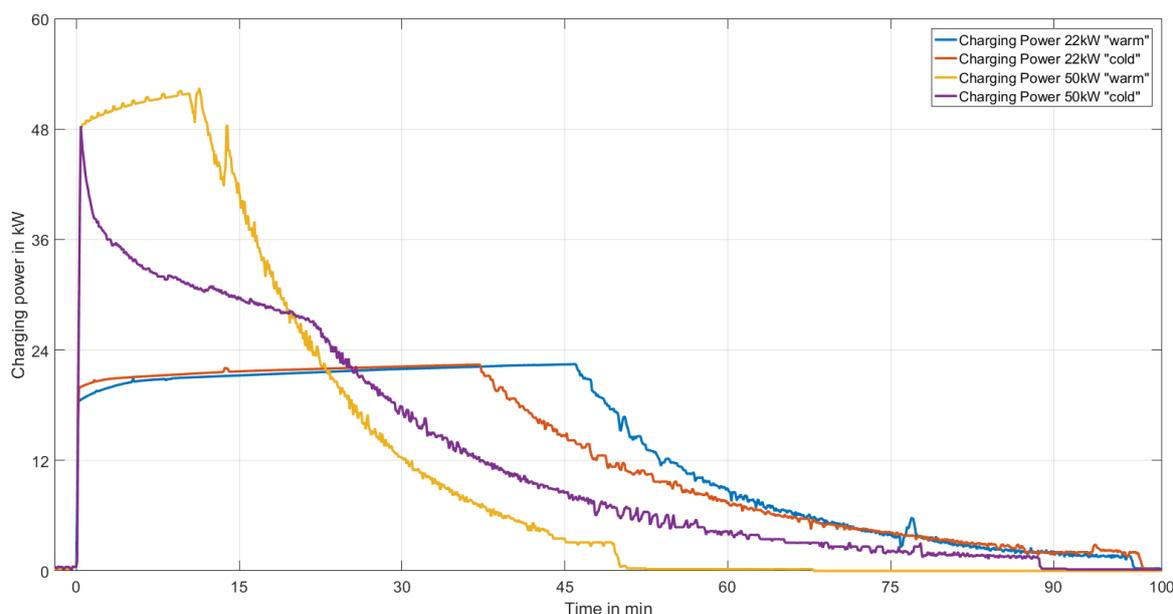
Figure 11: Comparison of various full charging profiles with a Nissan Leaf (different charging power and battery temperatures)
