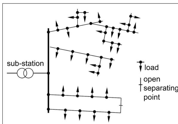
Figure 5: Grid topology - radial network (upper feeder) and open ring (lower feeder)[5]
