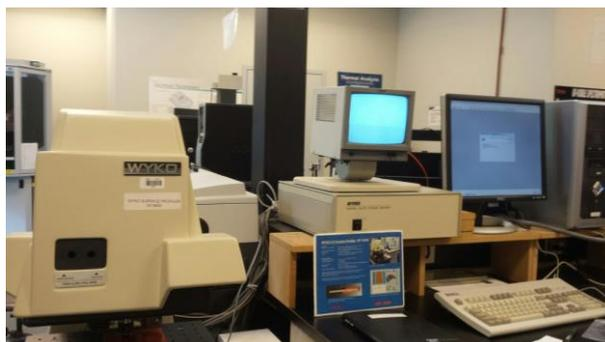
Figure 3 Picture of the optical surface profiler (WYKO) system
