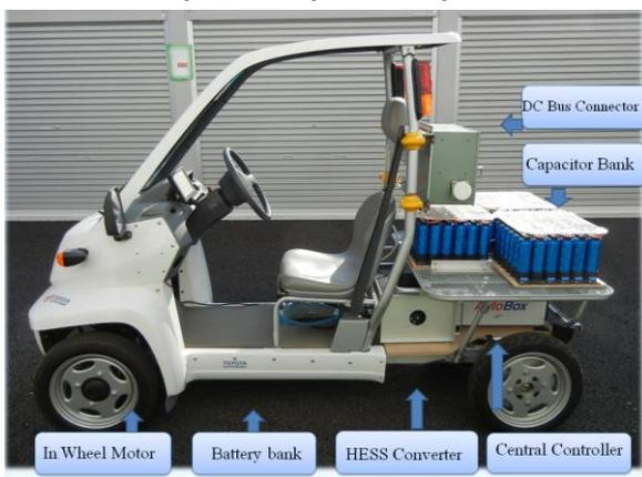
Fig. 2: Hybrid Electric Vehicle Prototype
