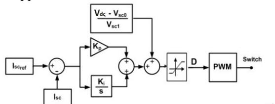
Fig. 8. Main current control loop for Half Controlled converter [7]
