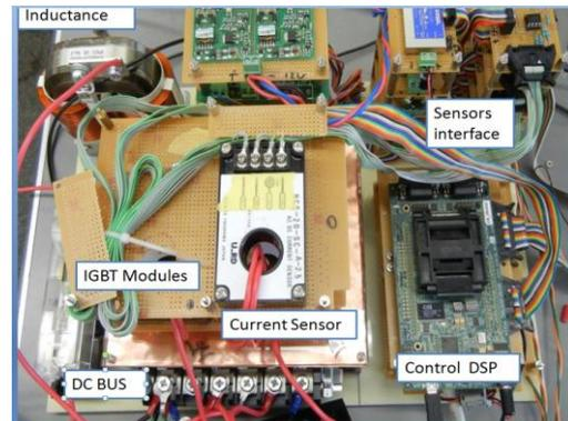
Fig.6. Converter Prototype for SC power interface
