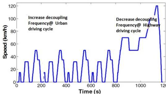
Fig 6 NEDC speed profiles from ref. [6]
