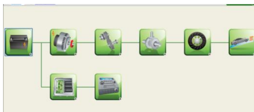
Figure 5: Propulsion Architecture without multi-gearbox
