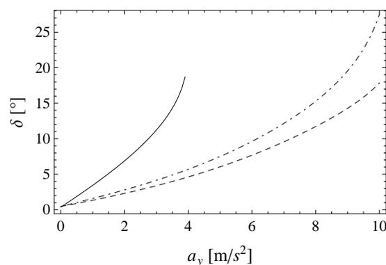
Figure 4: The steering-wheel angle  $\delta$  [°] as a function of the lateral acceleration  $a_y$  [m/s<sup>2</sup>] for the three torque distribution strategies, evaluated at a value of the longitudinal acceleration  $a_x = 5$  m/s<sup>2</sup>. The solid curve refers to strategy i), the dashed curve refers to strategy ii), and the dot-dashed curve refers to strategy iii).
