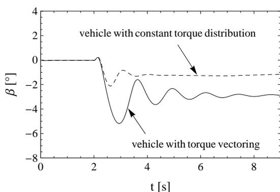
Figure 9: Step steer response ( $0^\circ$ - $100^\circ$ ) evaluated at  $a_x=3 \text{ m/s}^2$  and  $V=90 \text{ km/h}$ . The dashed curve refers to a vehicle with a constant torque distribution whereas the black curve refers to a torque vectoring strategy that consists in the torque distribution proportional to the vertical load acting on the wheel
