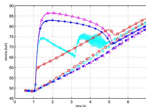
Figure13: Wheel (continuous line) and vehicle velocities (dashed line) during a tip-in manoeuvre. Vehicle without control system ( $\Delta$ ); vehicle with traction control based on a proportional gain (\*); vehicle with traction control based on a PID (Proportional-Integral-Derivative) controller ( $\square$ ); vehicle with traction control based on a proportional gain and the novel half-shaft torque control (o)
