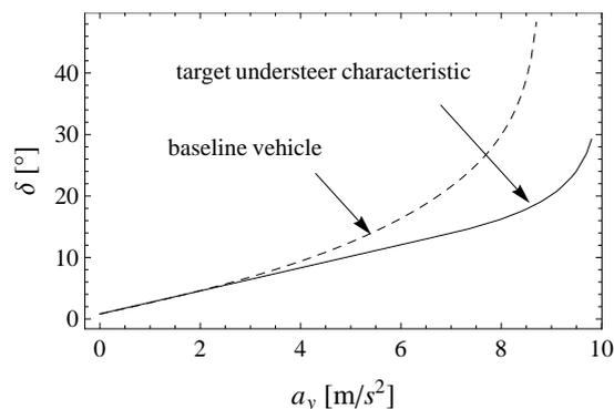
Figure 6: The understeer characteristic of the baseline vehicle (dashed line) and the desired understeer characteristic (solid line) evaluated at  $V=90$  km/h and  $a_x=2$  m/s<sup>2</sup>
