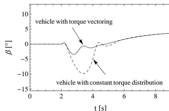
Figure 10: Step steer response ( $0^\circ$ - $100^\circ$ ) evaluated at  $a_x=-3 \text{ m/s}^2$  and  $V=90 \text{ km/h}$ . The dashed curve refers to a vehicle with a constant torque distribution whereas the black curve refers to a torque vectoring strategy that consists in the torque distribution proportional to the vertical load acting on the wheel
