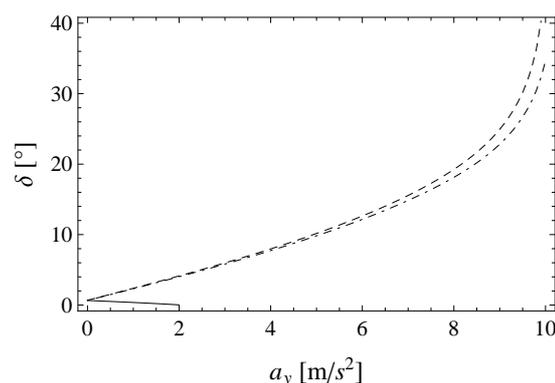
Figure 5: The steering-wheel angle  $\delta$  [°] as a function of the lateral acceleration  $a_y$  [m/s<sup>2</sup>] for the three torque distribution strategies, evaluated at a value of the longitudinal acceleration  $a_x = -5$  m/s<sup>2</sup>. The solid curve refers to strategy i), the dashed curve refers to strategy ii), and the dot-dashed curve refers to strategy iii).
