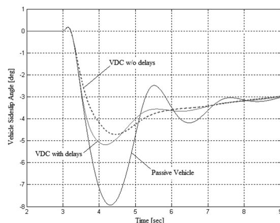
Figure 11: Comparison of vehicle response (vehicle sideslip angle) during step steer for a passive vehicle, a vehicle including an ideal VDC without delays in the actuation system, and a vehicle actuated by a commercial VDC unit (HIL test)
