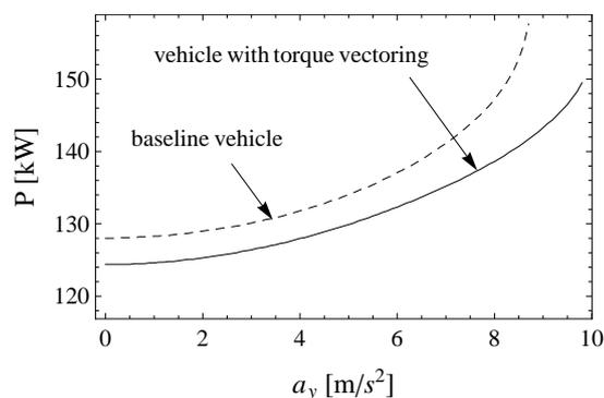
Figure 7: The overall motor input power  $P$  [kW] as a function of lateral acceleration  $a_y$  [m/s<sup>2</sup>], evaluated for the baseline vehicle (dashed line) and for the vehicle with torque vectoring (solid line) at  $V=90$  km/h and  $a_x=2$  m/s<sup>2</sup>
