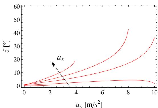
Figure 3: The steering-wheel angle  $\delta$  [°] as a function of the lateral acceleration  $a_y$  [m/s<sup>2</sup>], considering a constant torque distribution for different values of the longitudinal acceleration  $a_x$  [m/s<sup>2</sup>], from  $a_x = -5$  m/s<sup>2</sup> to  $a_x = 5$  m/s<sup>2</sup> in steps of 2.5 m/s<sup>2</sup>
