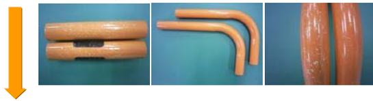
After salt spray test: No further spread of paint and peeling.
