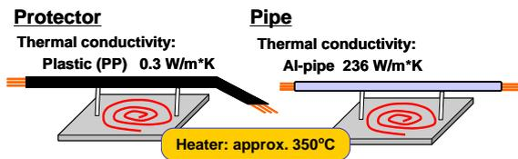
Figure 6: The test setup ability to transfer the heat in axial direction of the wiring harness
