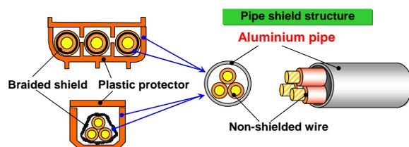
Figure 5: The concept of pipe shield wiring harness
