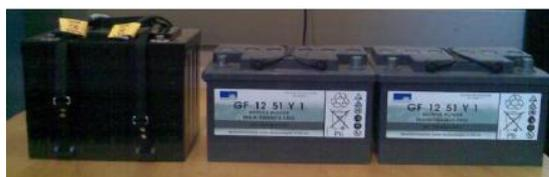
Figure 5 – Comparison between the dimensions of a lithium iron phosphate battery (left) and an equivalent lead acid battery (right)
