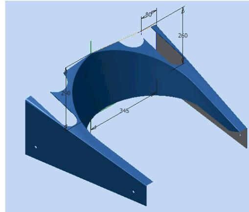
Figure 15: Back middle piece drawn in surface modelling
