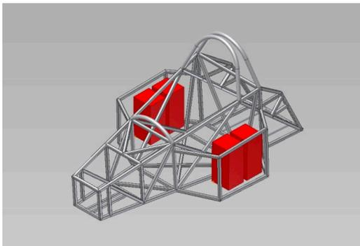
Figure 10: Placement of the batteries
